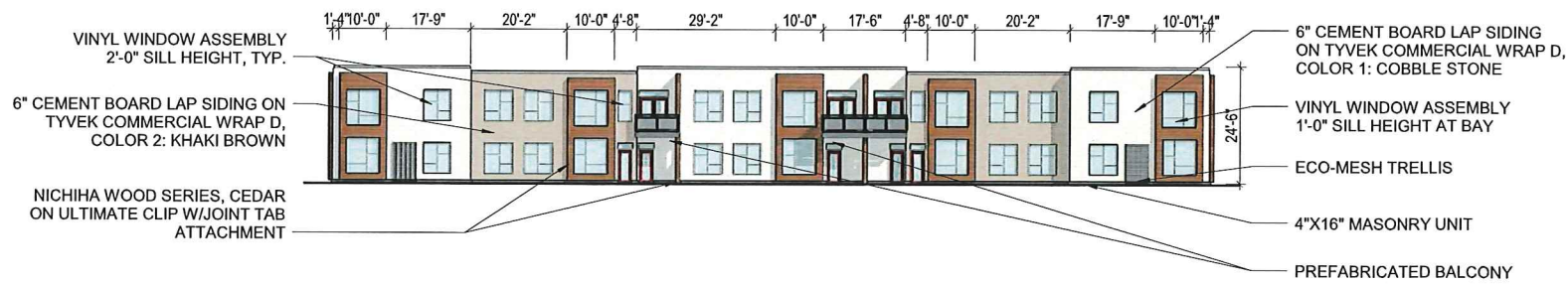
BUILDING A1/A2 - EAST ELEVATION
