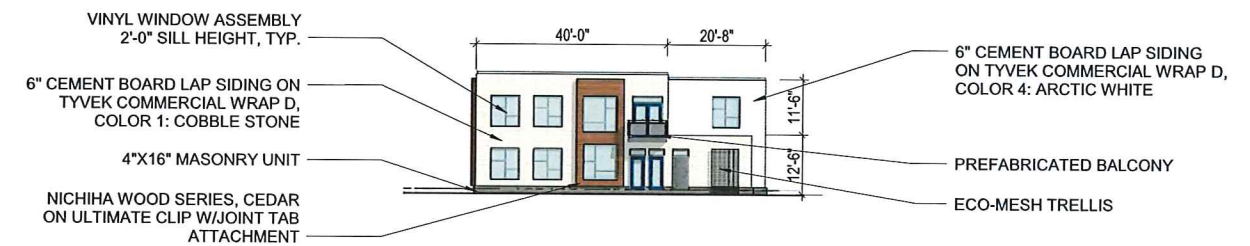
BUILDING B2/B3 - EAST ELEVATION
