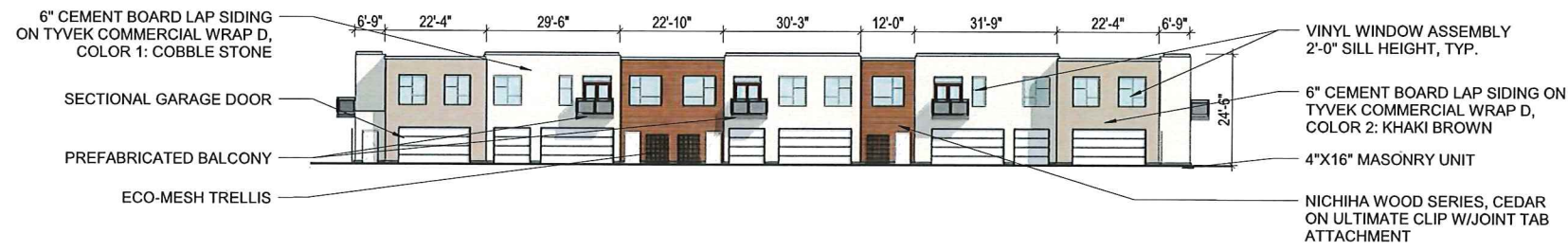
BUILDING A1/A2 - WEST ELEVATION
