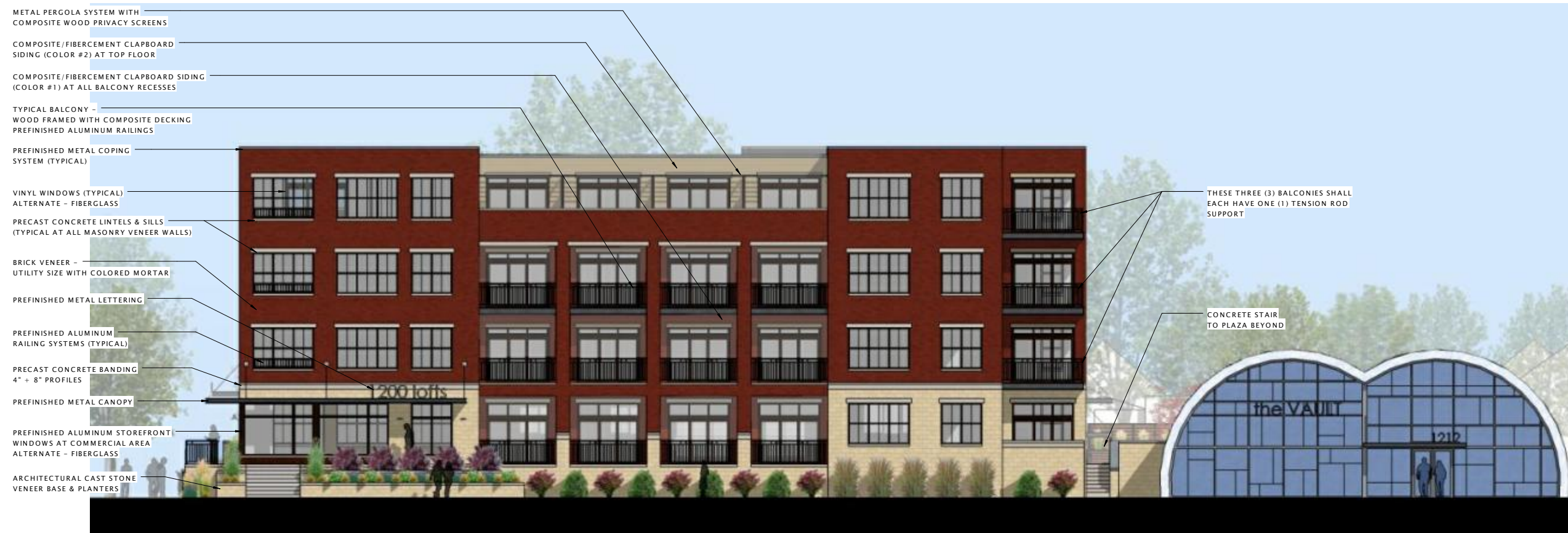
⑥ EAST WASHINGTON AVENUE ELEVATION 1/8" = 1'-0"
