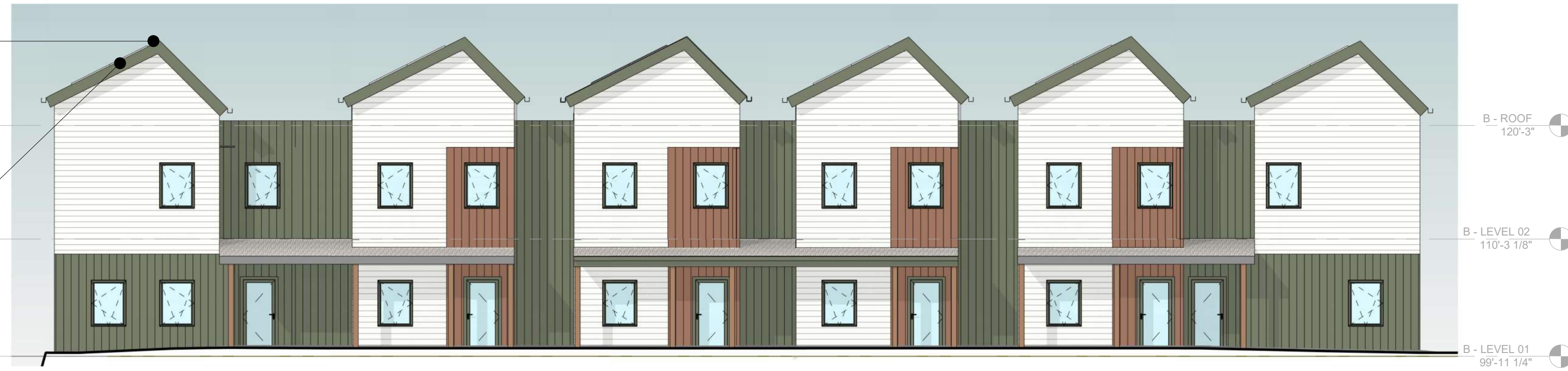
3A EXTERIOR ELEVATION - SOUTH 1/8" = 1'-0"
