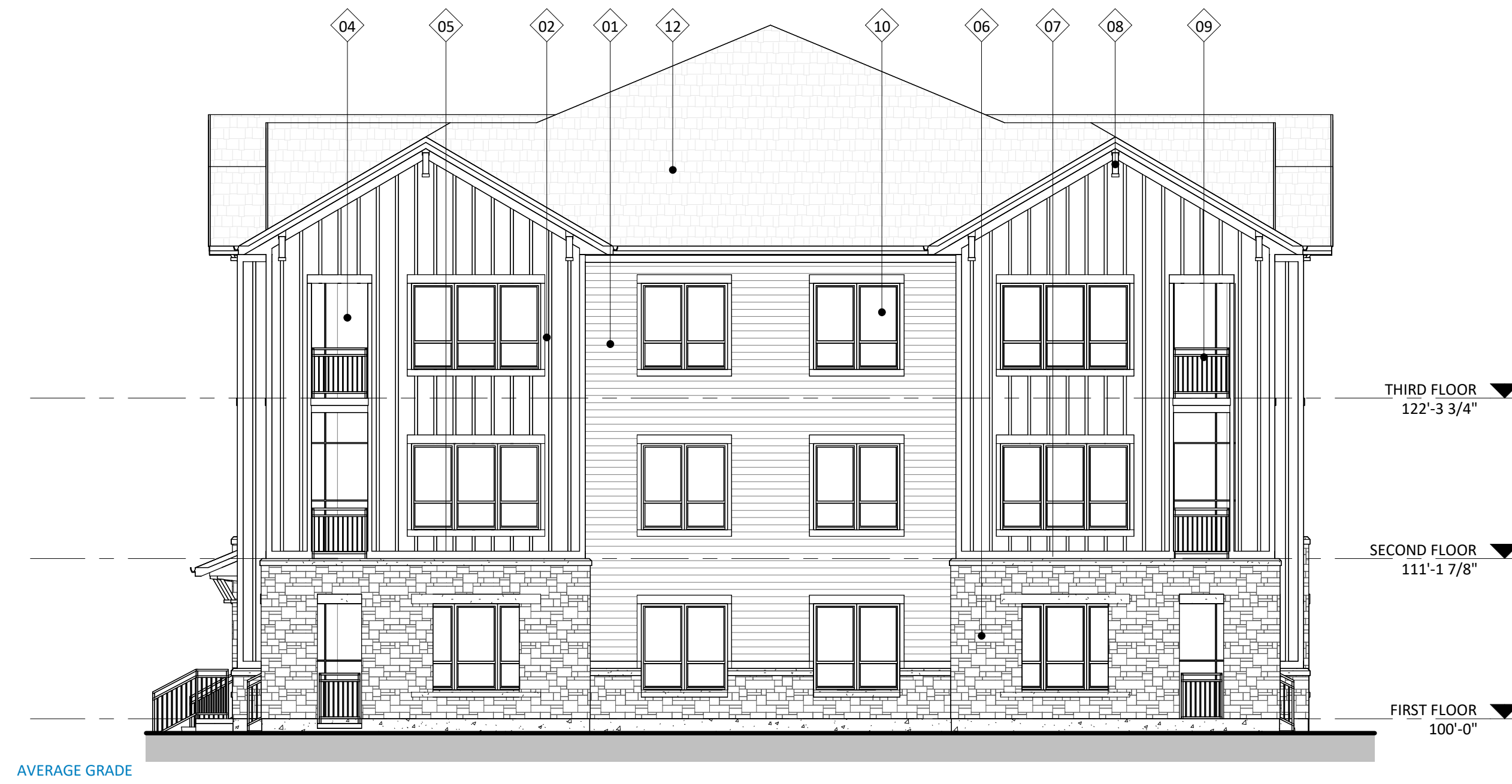
2 ELEVATION - NORTHWEST AC201-5 1/8" = 1'-0"
