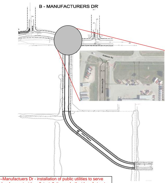
~Manufactuers Dr - installation of public utilities to serve development, sidewalk installation on both sides of street from existing street to north boundary of CSM Lot 2 ~North of CSM Lot 2, Manufactuers Dr will be one way northbound with a narrowed roadway at the intersection with Anderson Rd.
