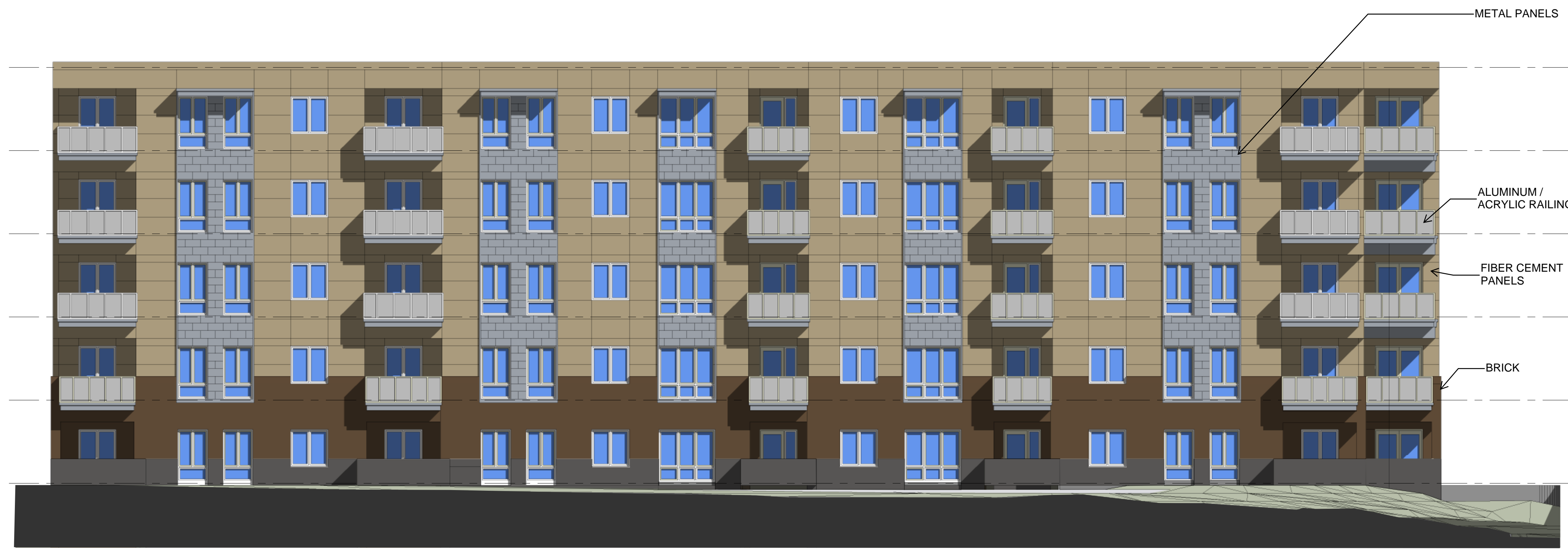
1 Independent Living - West Elevation SCALE: 1/8" = 1'-0"
