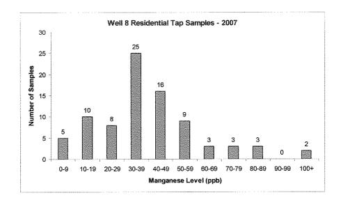
**Recommendation**: Staff does not recommend that the Board take any action at this time. UW 8 should be considered as problematic because of the potential for colored water. Dependent on the outcome of the location of a replacement site for UW 3, UW 8 may be a candidate for future filtration for manganese and iron.
