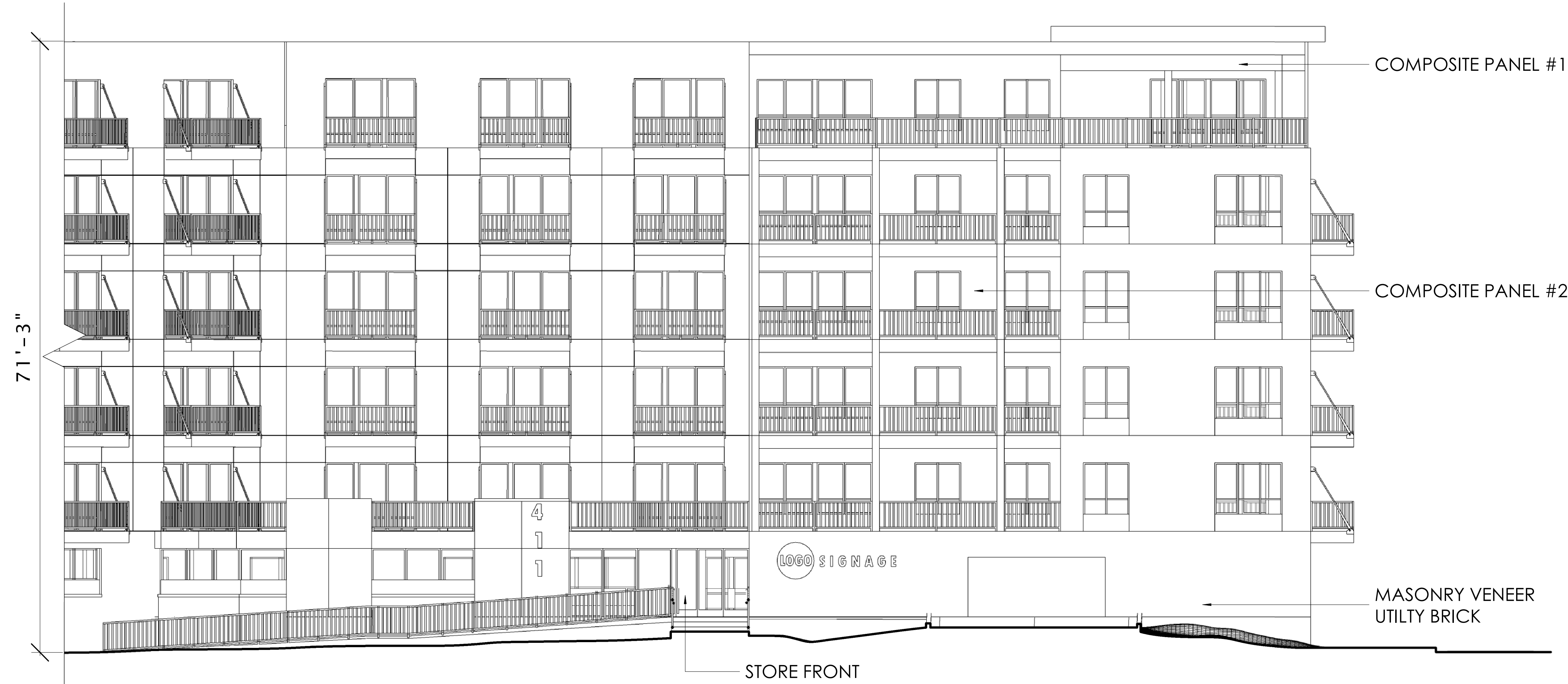
1 NORTHEAST ELEVATION B&W 1/8" = 1'-0"
