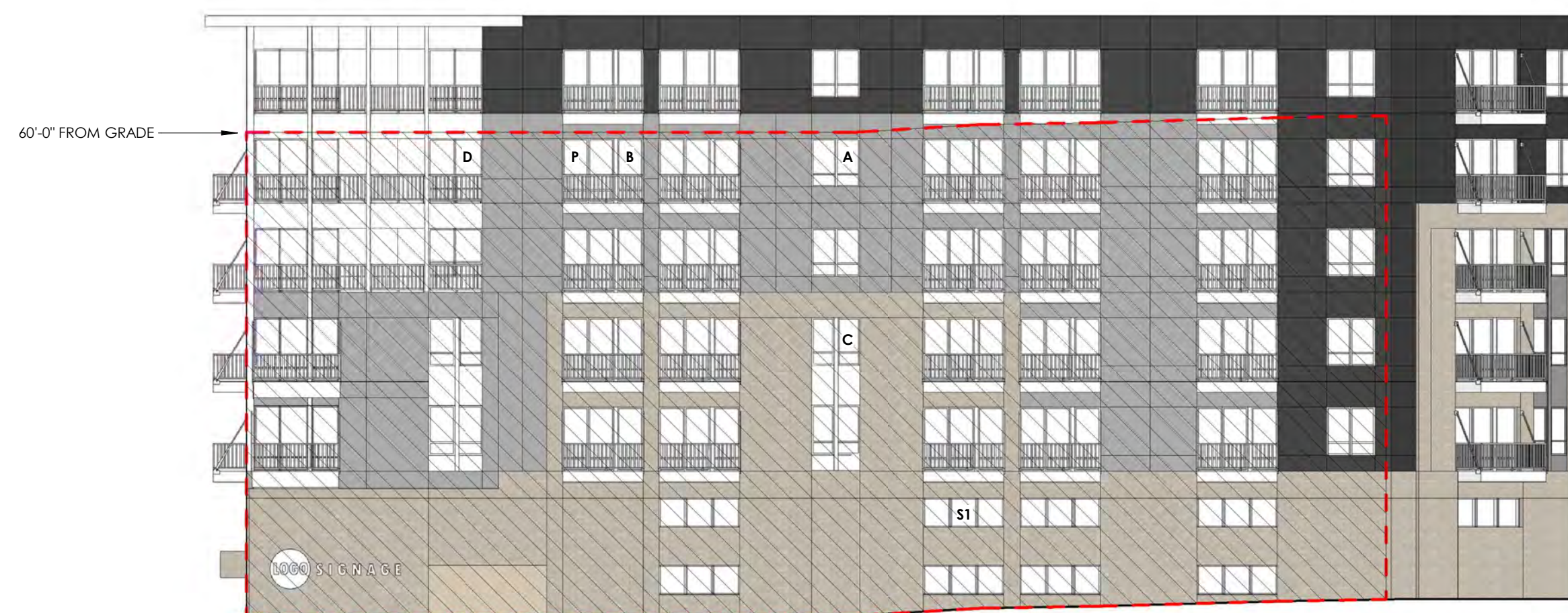
⑰ SOUTHWEST ELEVATION BIRD GLASS 1/16" = 1'-0"
