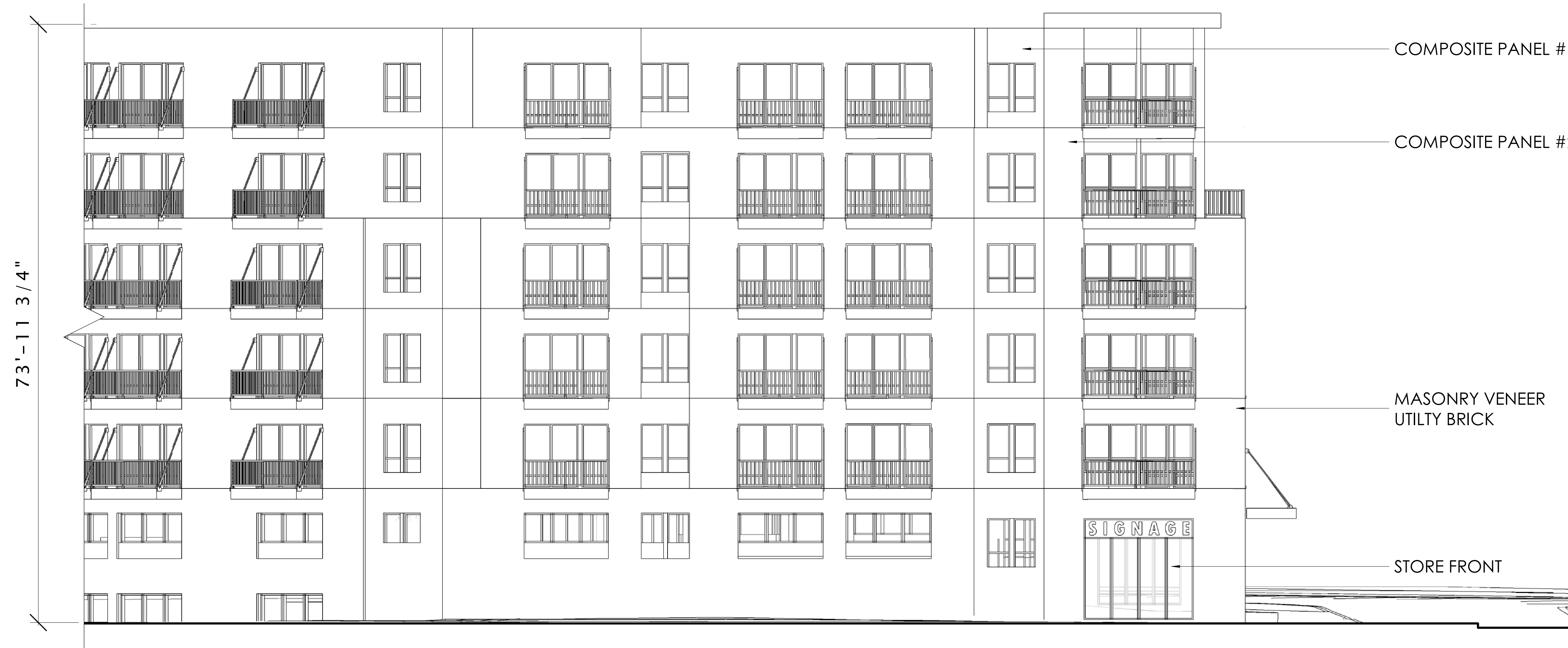
6 SOUTH ELEVATION B&W 1/8" = 1'-0"
