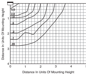
Isofootcandle plot of one 50W HPS E5 Up/Down Cutoff Light at 10' (3.0 m) mounting height (plan view).
