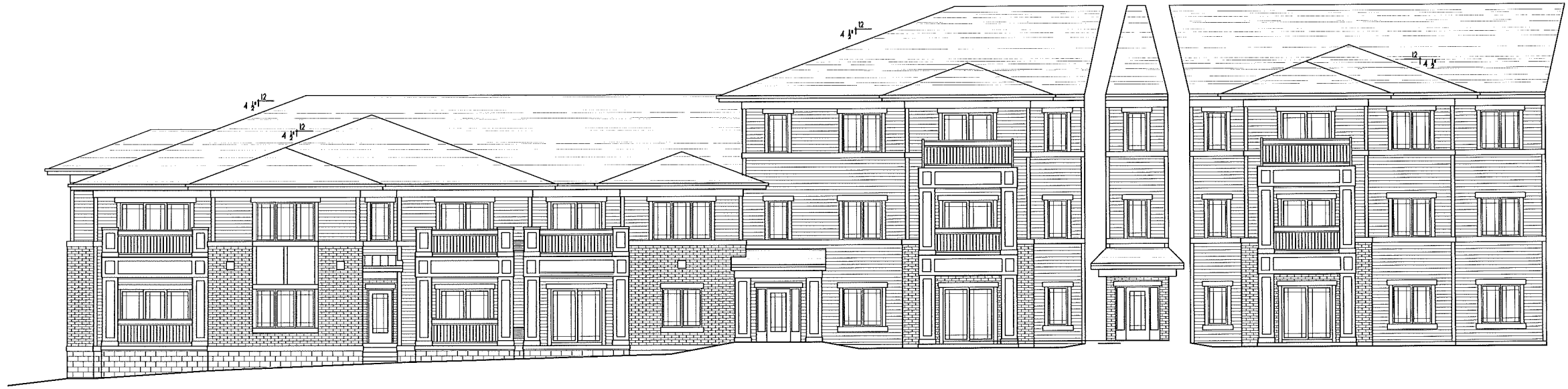
BUILDING A - INSIDE SOUTHWEST ELEVATION SCALE - 1/8" = 1'-0"
