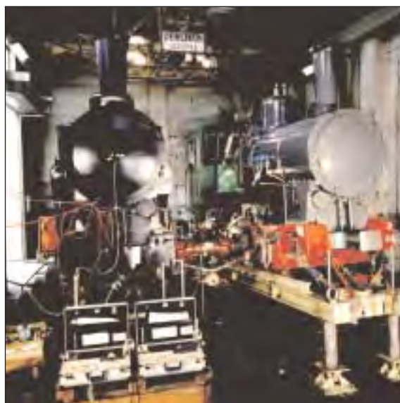
Fig. 10: Work load trials at SLM with locomotive No.12 of the Brien Rothorn Railway on the left side and 999.201 of the Austrian Federal Railway. The two bright cases in the foreground contain the emission analysers.
