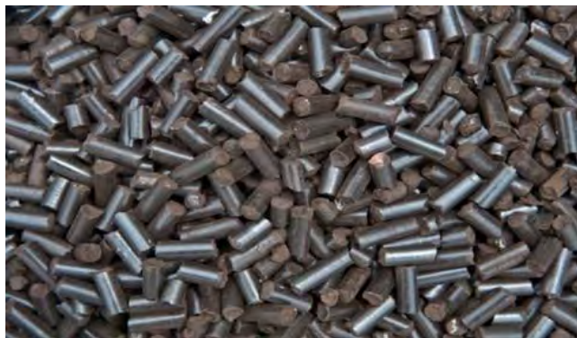
Figure 7. Hydrochar obtained in the HTC Ingelia process
