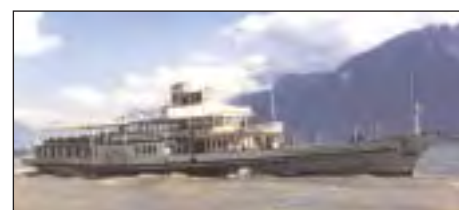
Fig. 24: The "Montreux" after conversion to diesel-electric drive, which improved the economics but certainly not the aesthetics.
