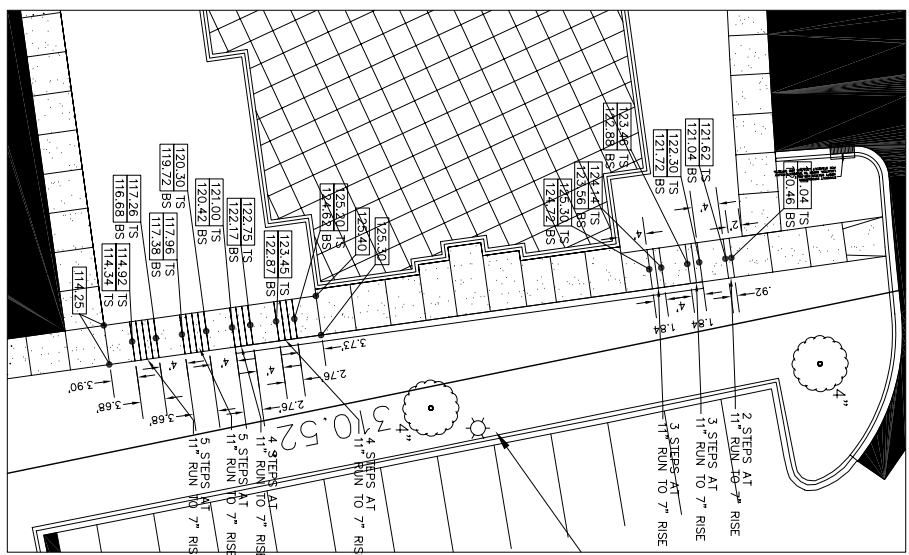
4 CONCRETE STAIR DETAIL 3 C1.2 NO SCALE
