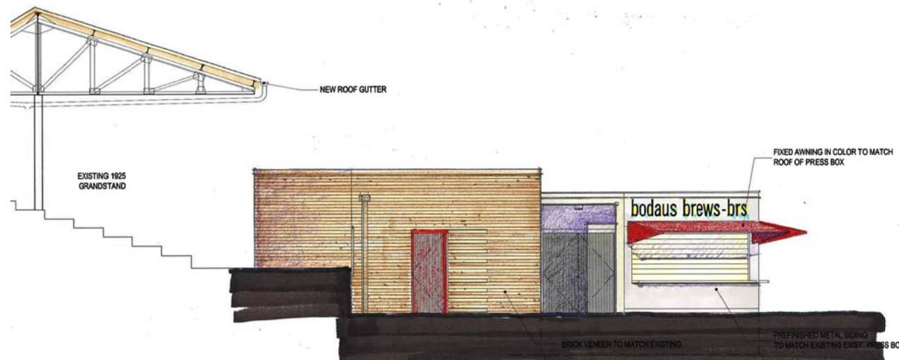
2 SOUTH ELEVATION - CONCESSIONS ADDITION Scale: 1/4"=1'-0"
