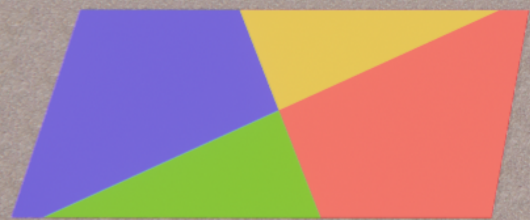
SHAPES CUT FROM 4' X 8' X 1/8" PERFORATED PANEL 2 PANELS PER EACH SHADE STRUCTURE
