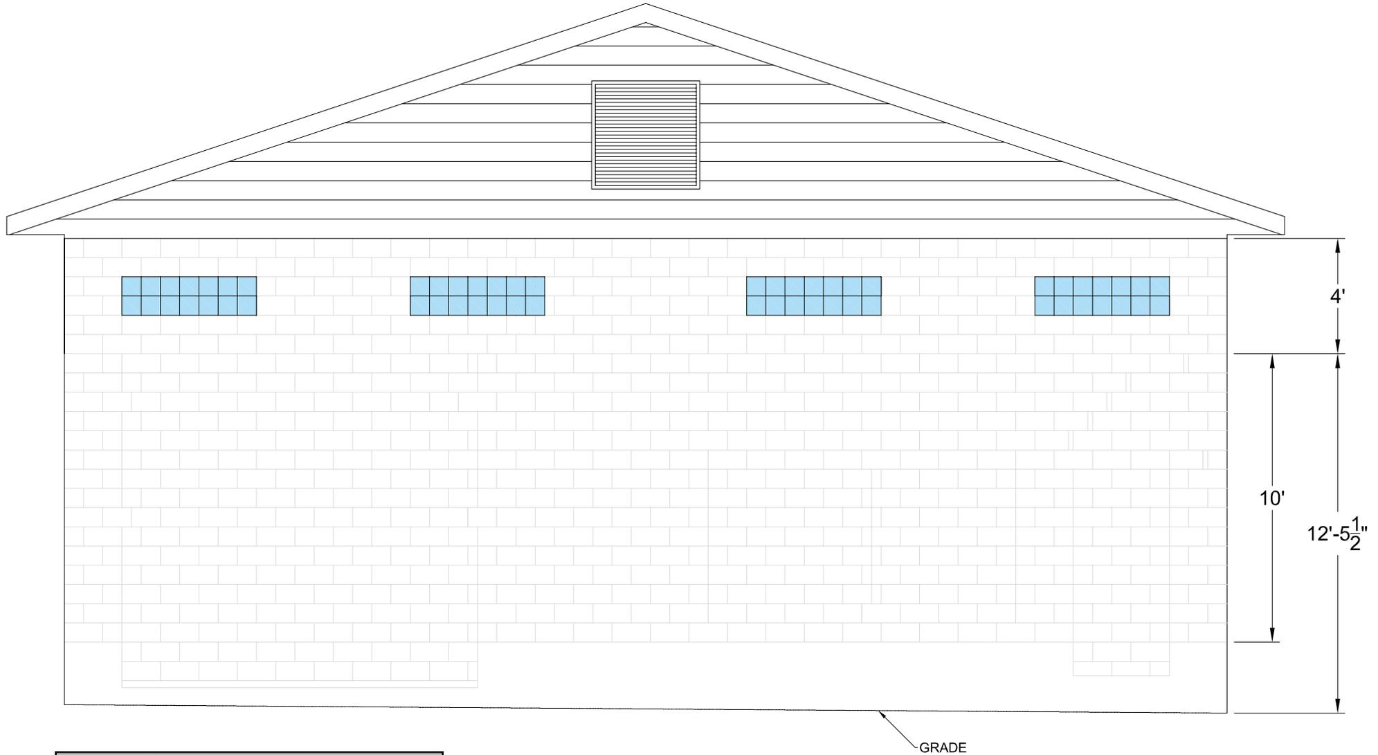
Drawing of East Elevation showing the proposed additional 4 feet of wall height and the roof addition. Glass block is planned to bring in natural light.
