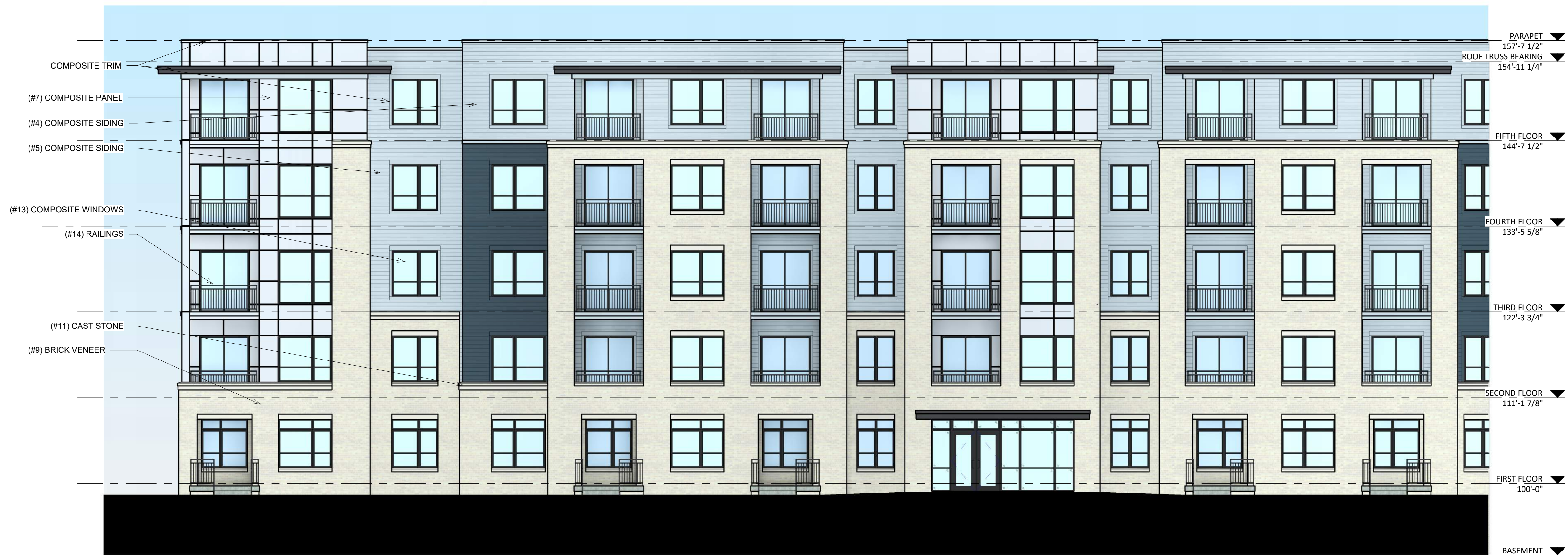
1 COLORED ELEVATION - BLDG 2 1.0 A201 1/8" = 1'-0"
