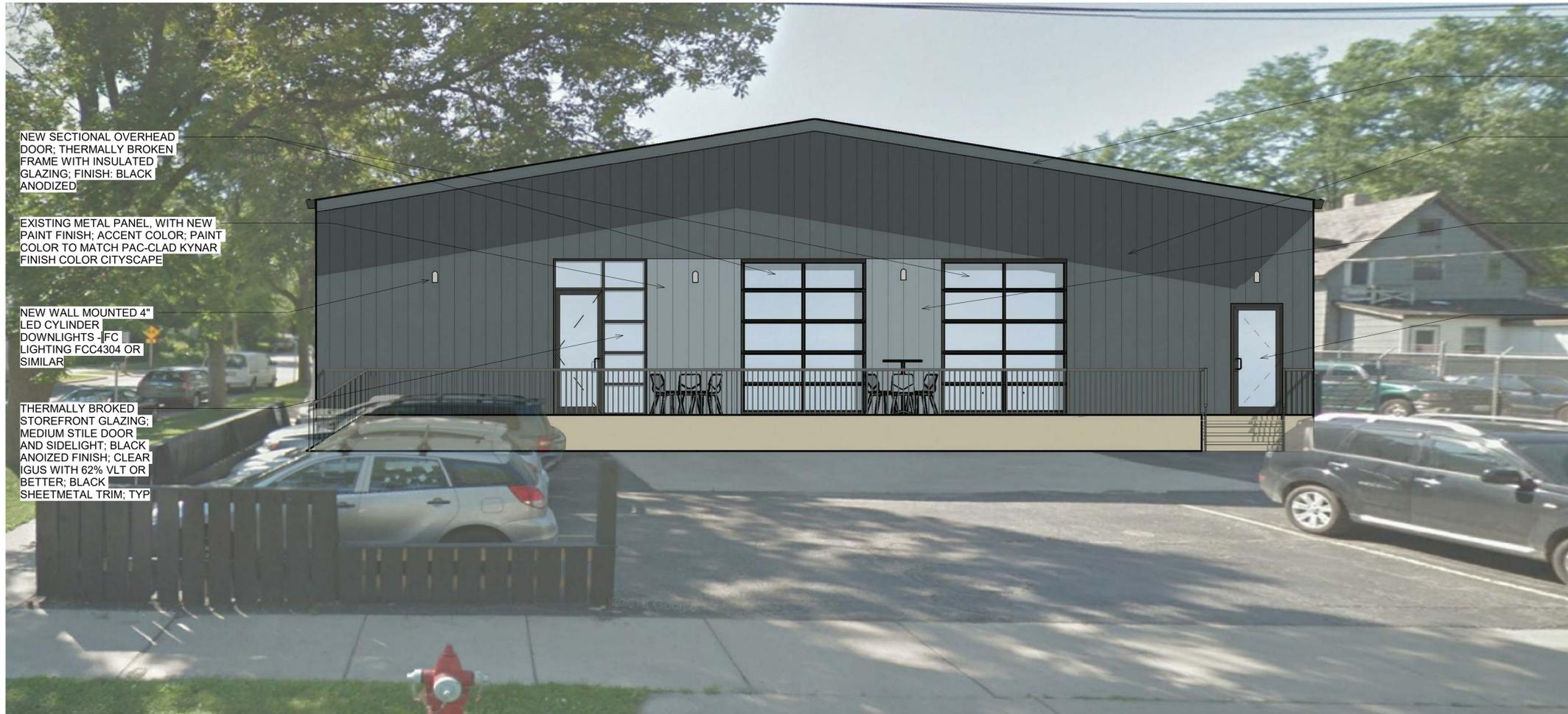
NEW SECTIONAL OVERHEAD DOOR; THERMALLY BROKEN FRAME WITH INSULATED GLAZING; FINISH: BLACK ANODIZED
