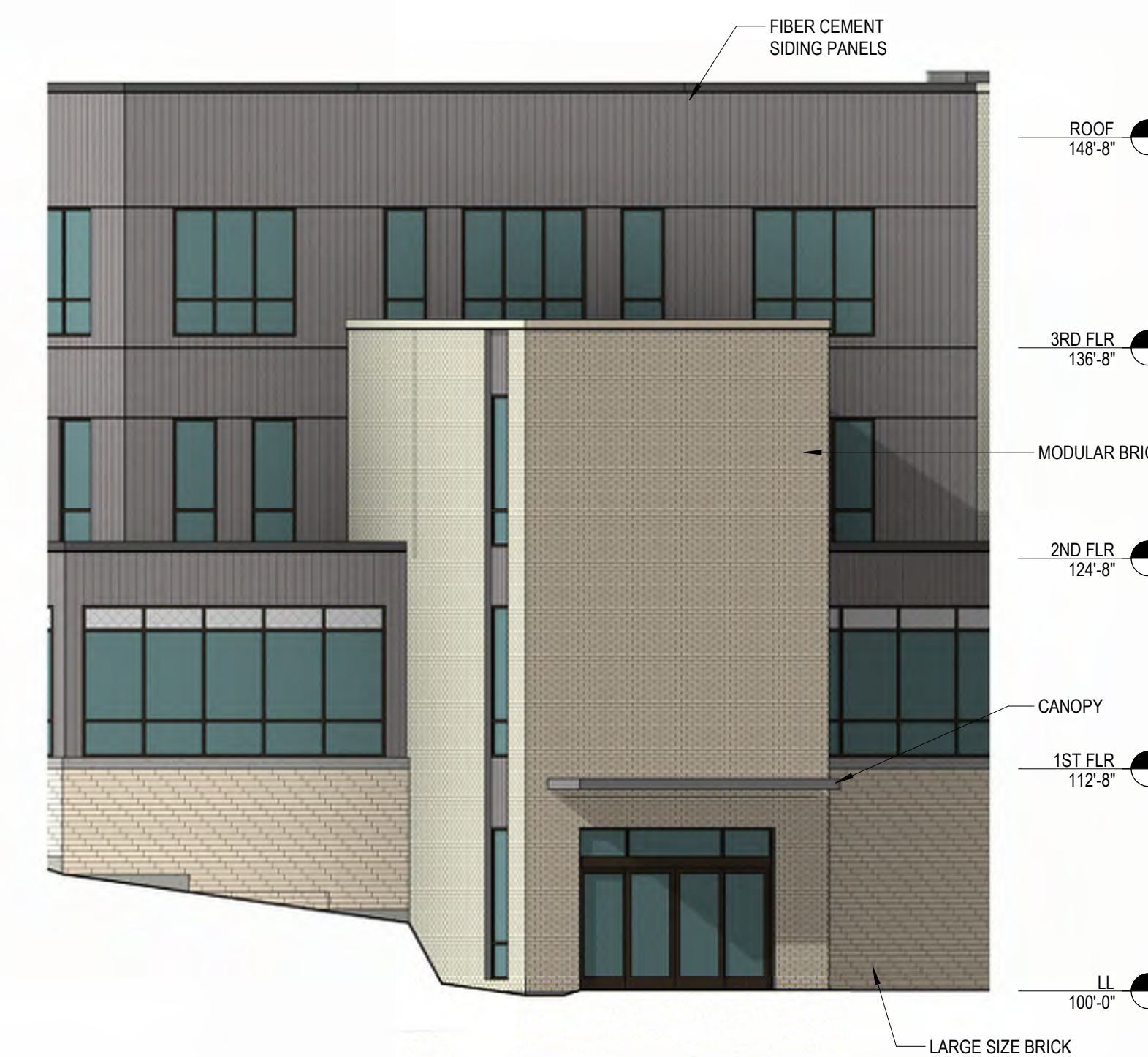
2 AREA C - NORTHEAST ELEVATION 1 1/8" = 1'-0"
