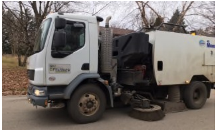
Figure 11-1. Street Sweeping Operations
