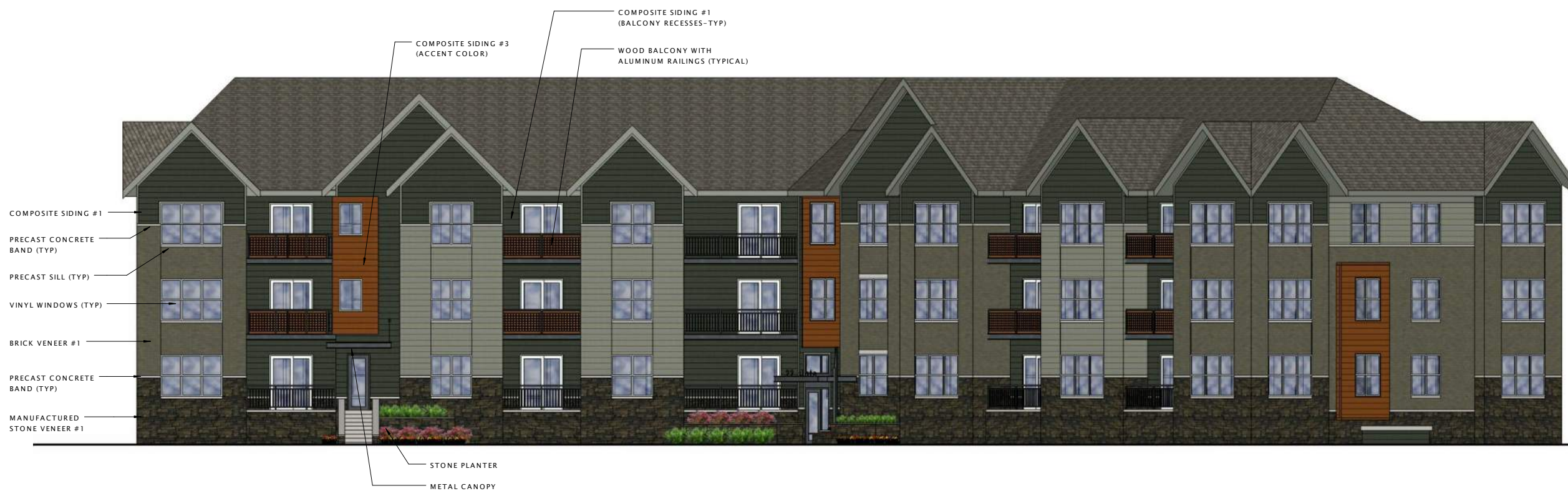
① B BLDG - North Elevation 1 1/8" = 1'-0"
