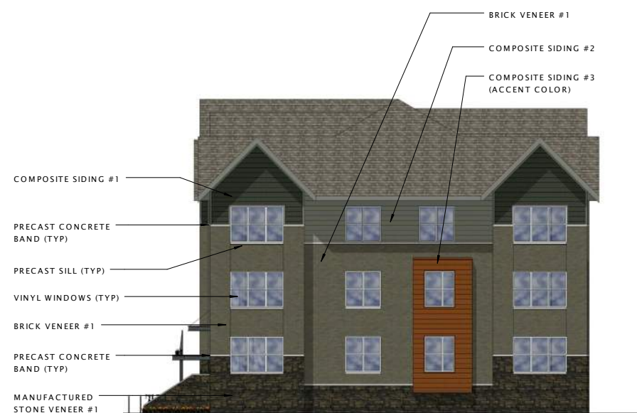
⑩ BUILDING 'A' - END ELEVATION 2 3/32" = 1'-0"
