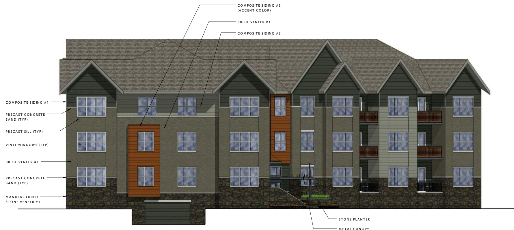
⑦ BUILDING 'B' - END ELEVATION 1 1/8" = 1'-0"
