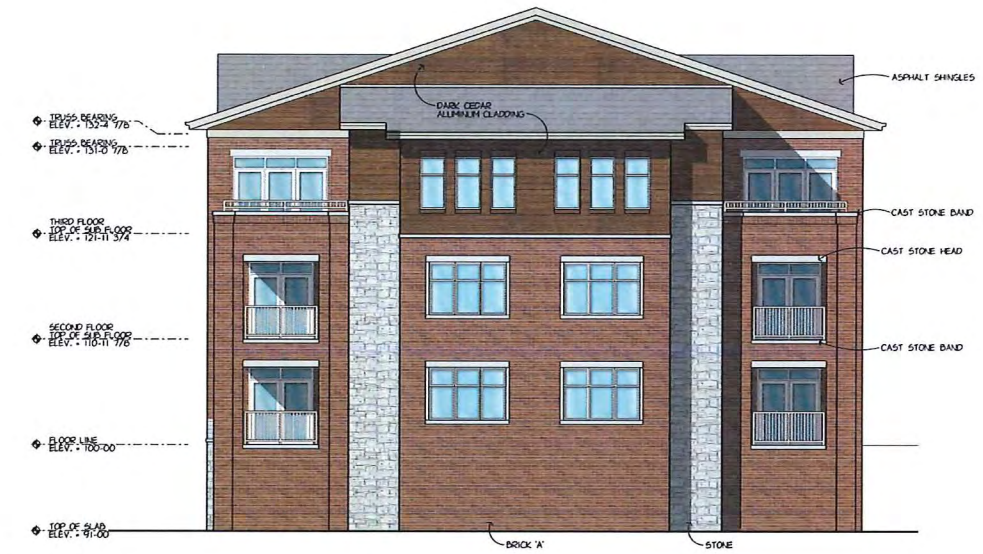
BUILDING 2: NORTH ELEVATION
