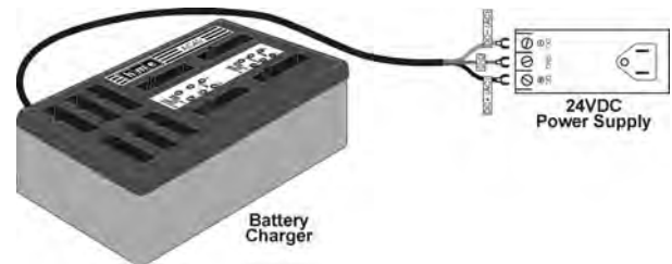
Figure 9. Battery charger power connection
