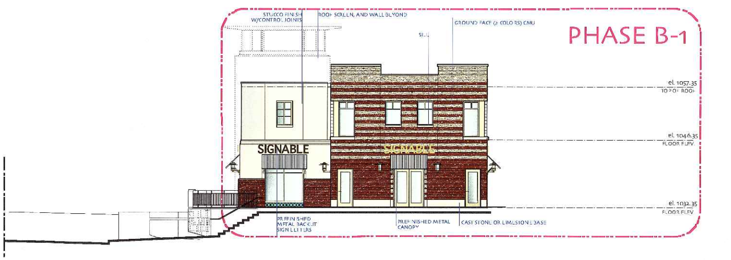
Phase B-1 South Elevation NOTE: Landscape not shown, see landscape plans for landscape information
