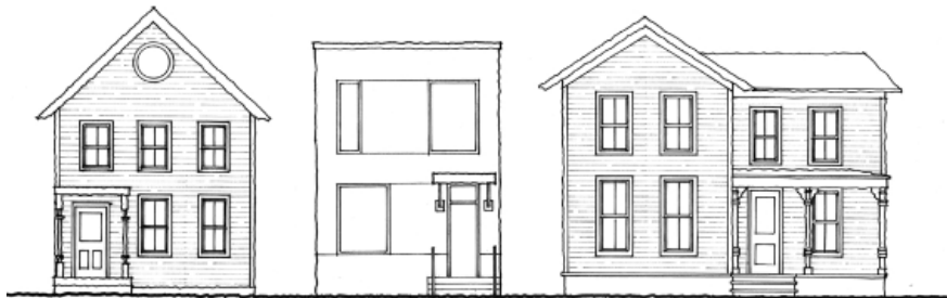
Inappropriate residential infill project which is not sensitive to the roof style, pattern and detailing of historic homes.
