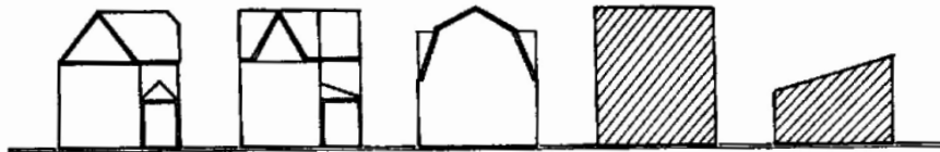
Roof shapes should be in harmony with surrounding historic buildings. Shaded structures are incompatible.
