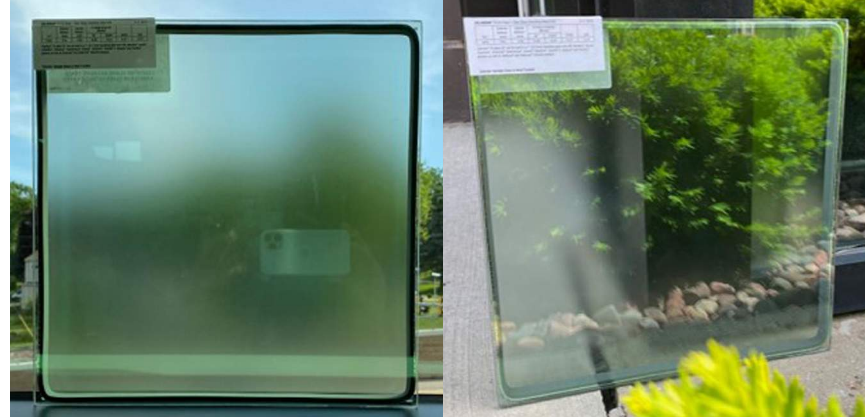
5 SOLARBAN 70 TRANSLUCENT GLASS SATINLITE 1 ON 3RD SURFACE (TO RECEIVE 2" X 4" BLACK BIRD GLAZING PATTERN)
