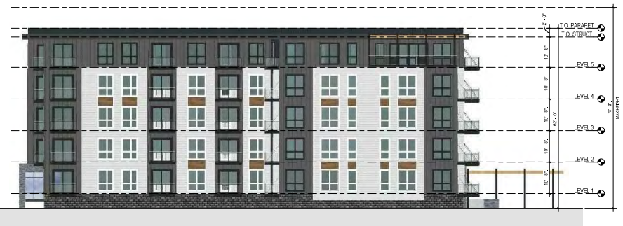
4 West Building - South Elevation 1/8" = 1'-0"
