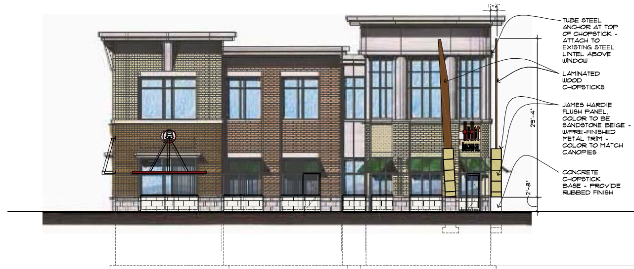
2 EXTERIOR SOUTH ELEVATION TD1.0 1/8" = 1'-0"
