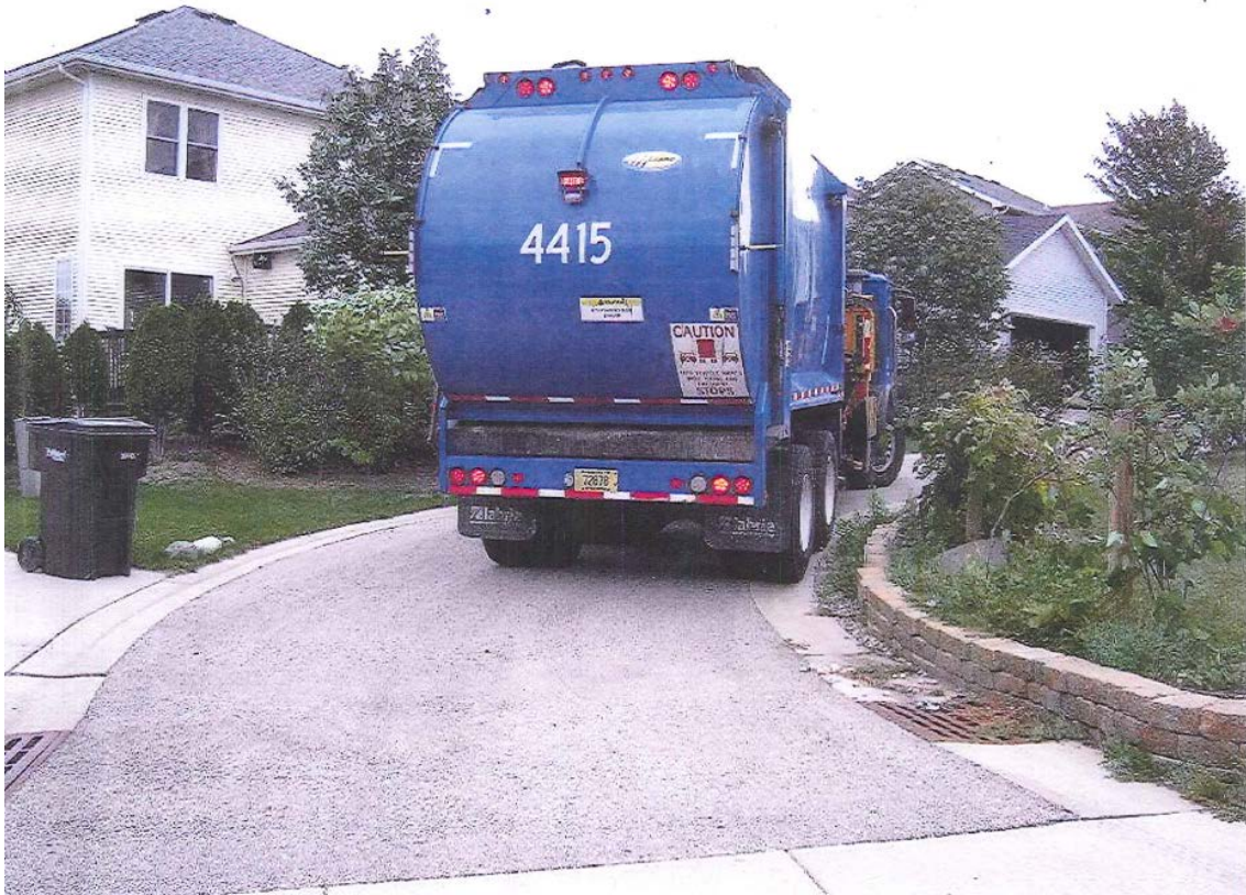
Landscaping encroaches into the right of way, which can cause damage to vehicles.
