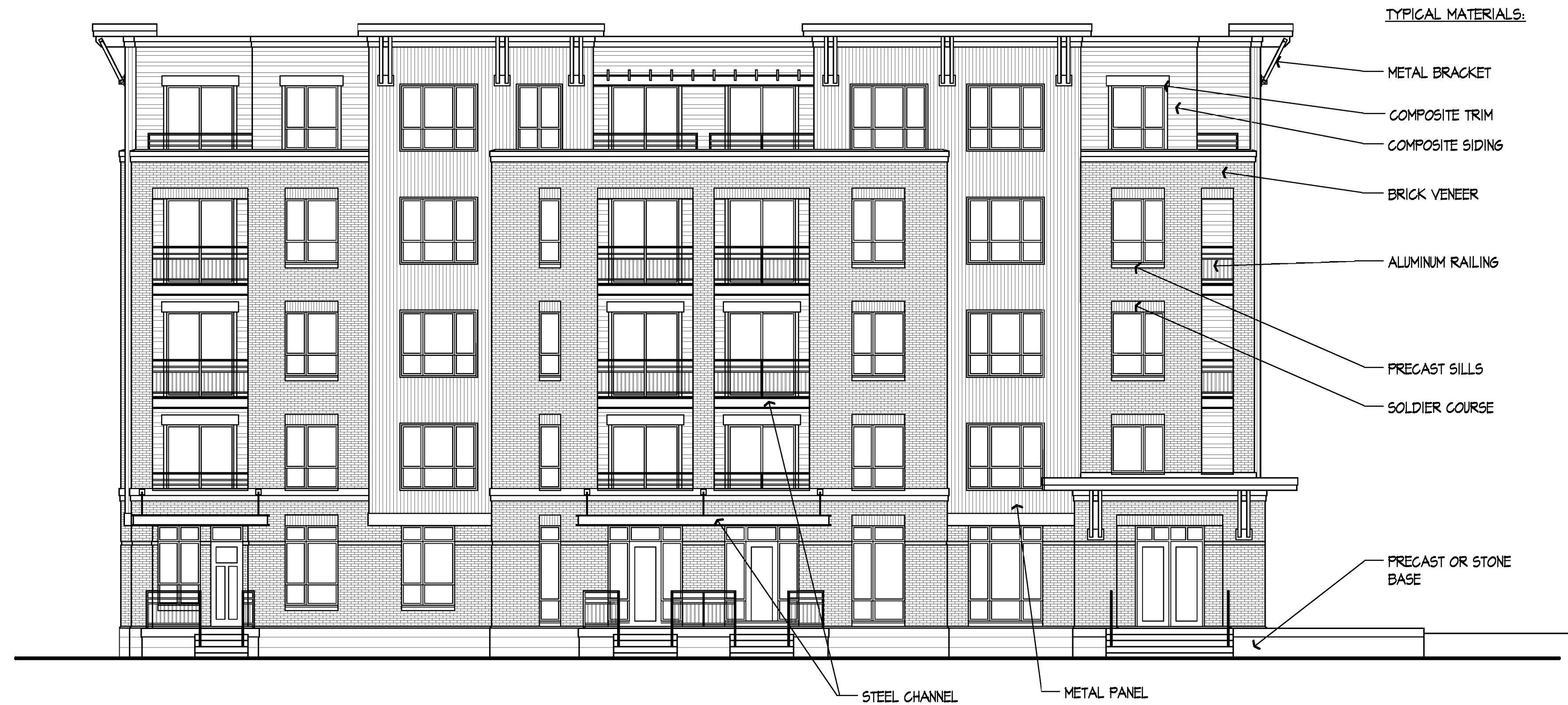
Bassett Street Elevation 1/8" = 1'-0"
