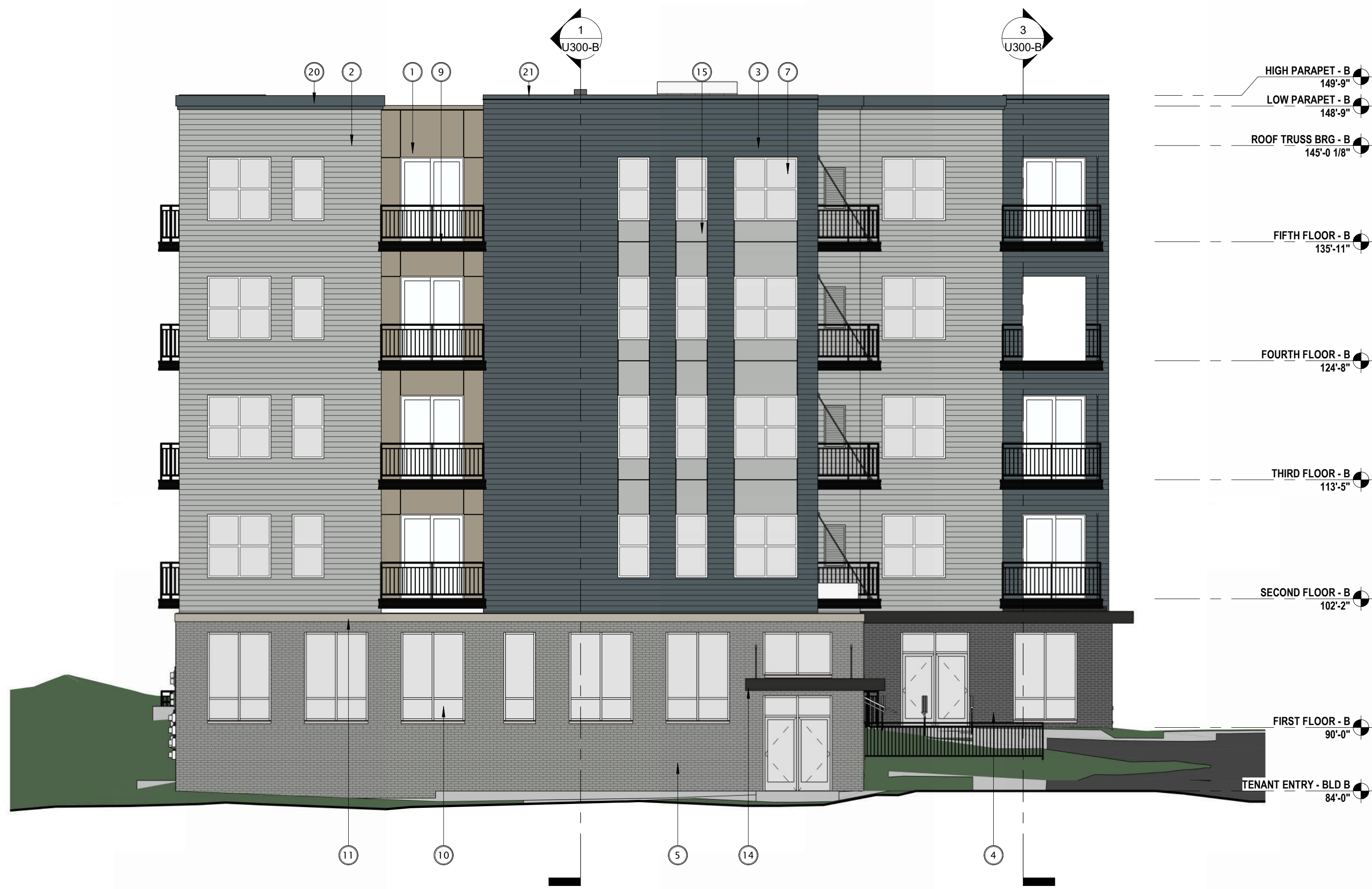
1 SOUTH ELEVATION - BUILDING B 1/8" = 1'-0"
