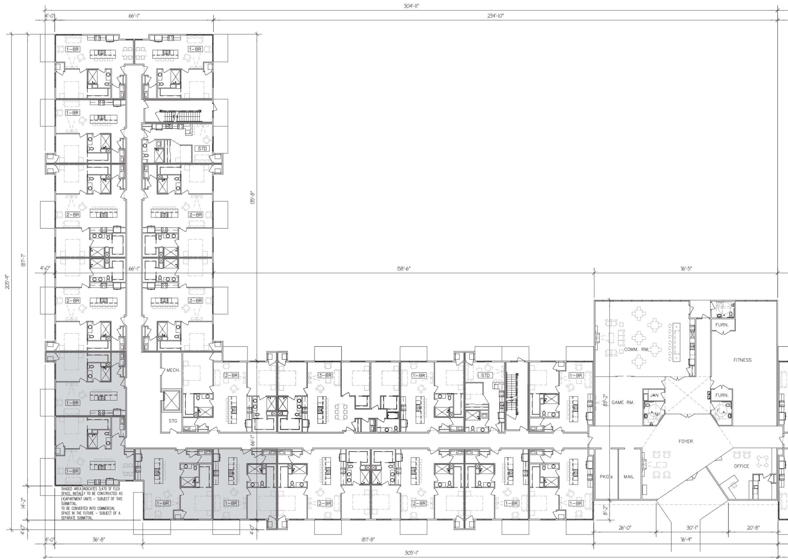
SHADED AREA INDICATES 3,470 SF FLEX SPACE, INITIALLY TO BE CONSTRUCTED AS (4) APARTMENT UNITS - SUBJECT OF THIS SUBMITTAL. TO BE CONVERTED INTO COMMERCIAL SPACE IN THE FUTURE - SUBJECT OF A SEPARATE SUBMITTAL.
