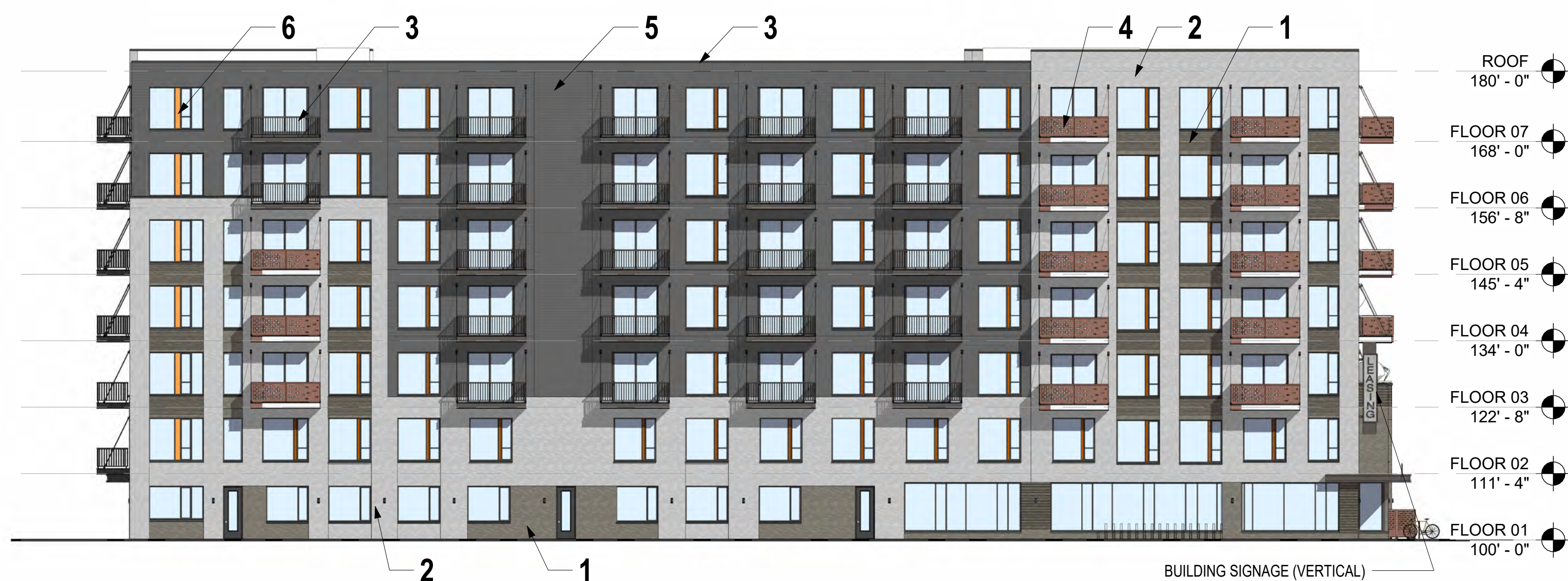
4 SOUTH ELEVATION A200 1/16" = 1'-0"
