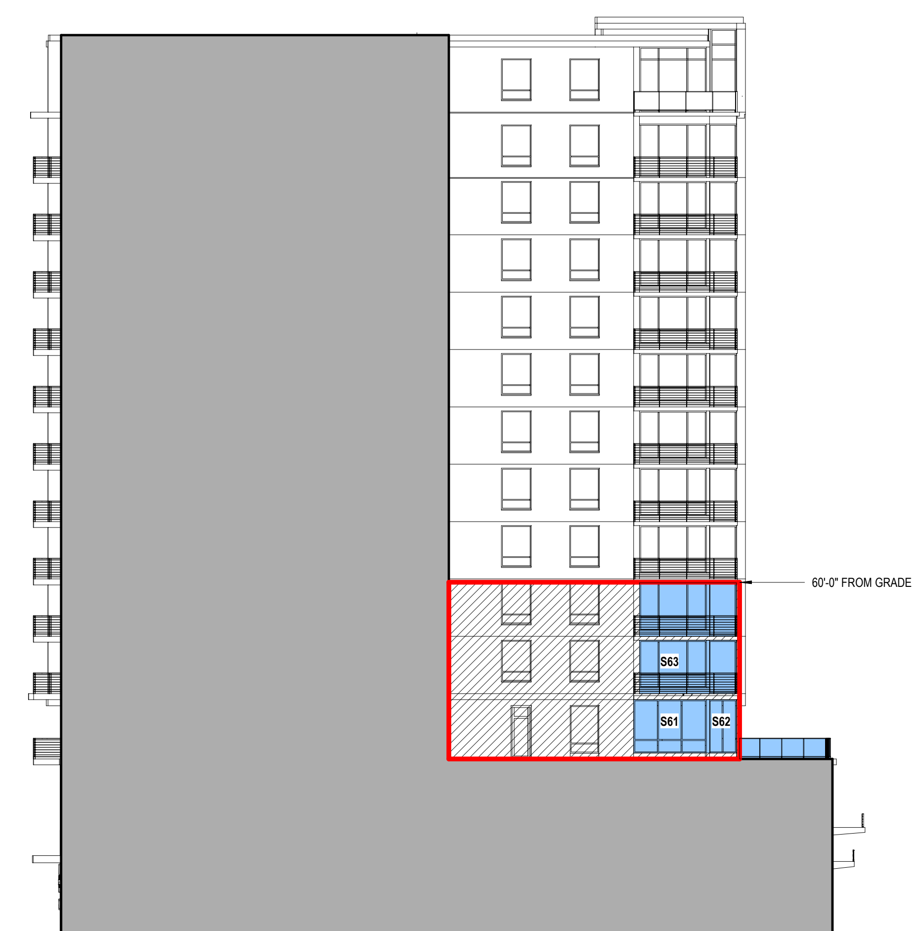
2 WEST ELEVATION BIRD-SAFE GLASS AUTOCAD 1/16" = 1'-0"
