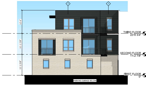
4 COURTYARD - WEST ELEVATION COLOR A-2.4 1/8" = 1'-0"
