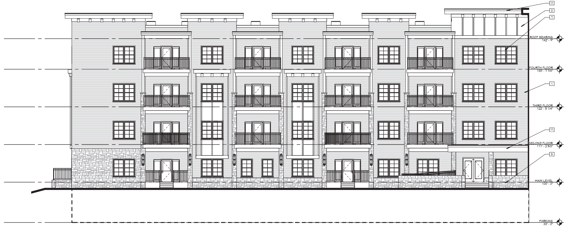
1 BUILDING 1 - NORTH ELEVATION (BLDG 2 SIM) A4.3 1/8" = 1'-0"
