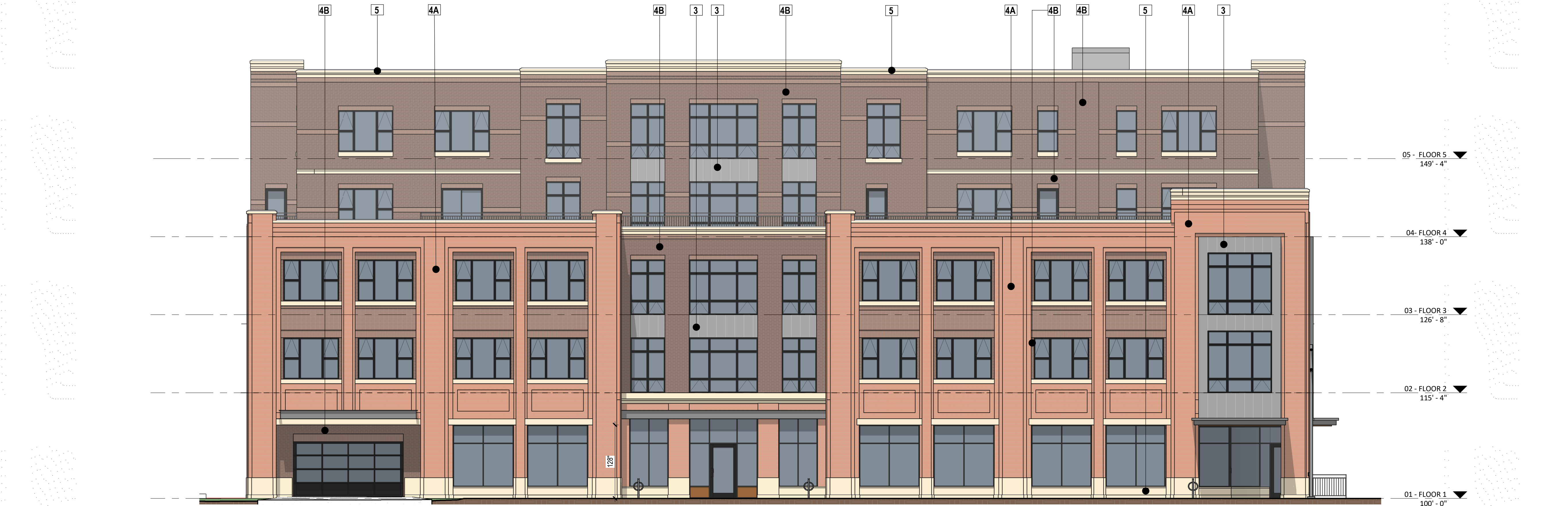
1 SE ELEVATION- WILLIAMSON ST- COLOR A2.3 1/8" = 1'-0"
