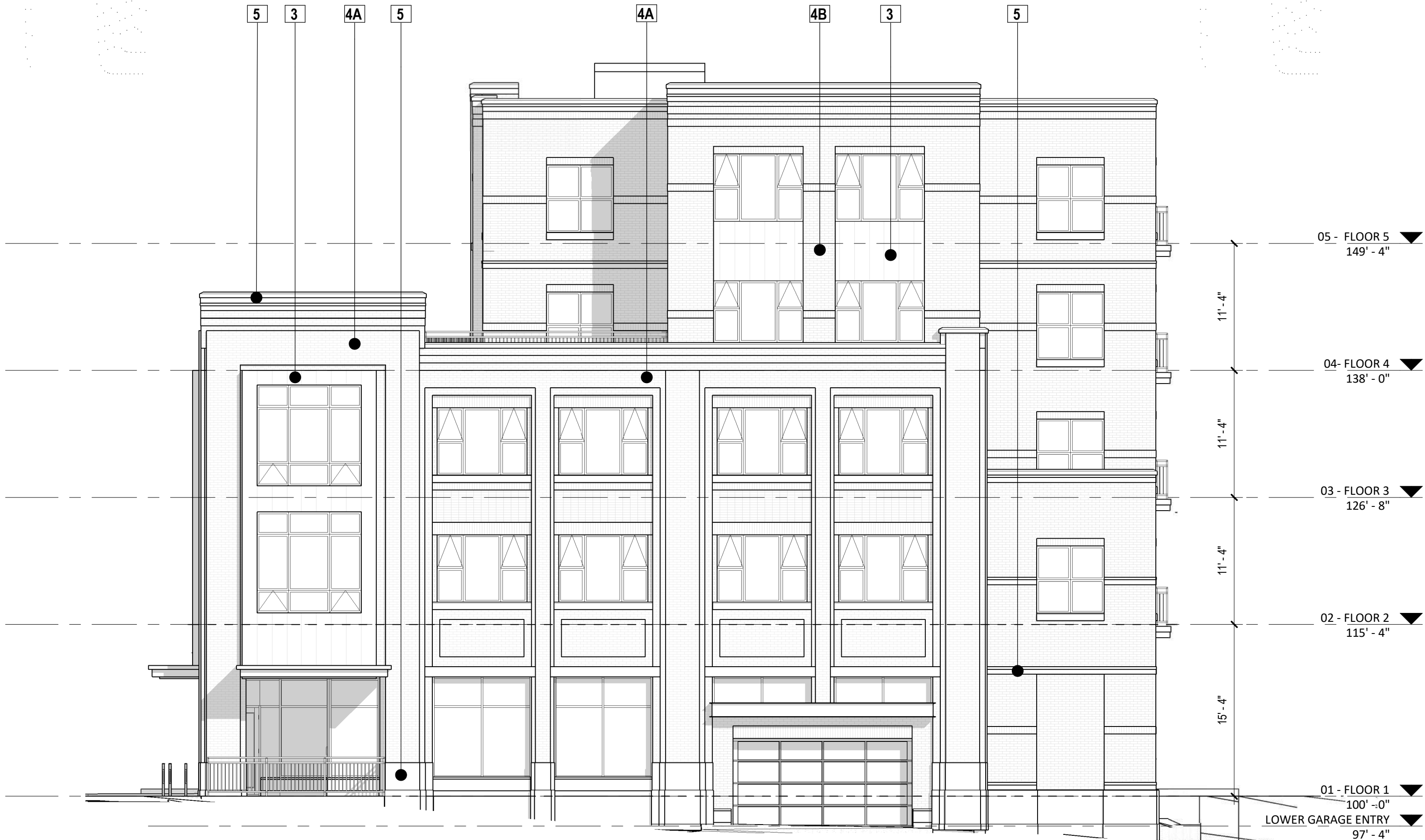
2 NE ELEVATION- S BLOUNT ST B&W A2.1 1/8" = 1'-0"
