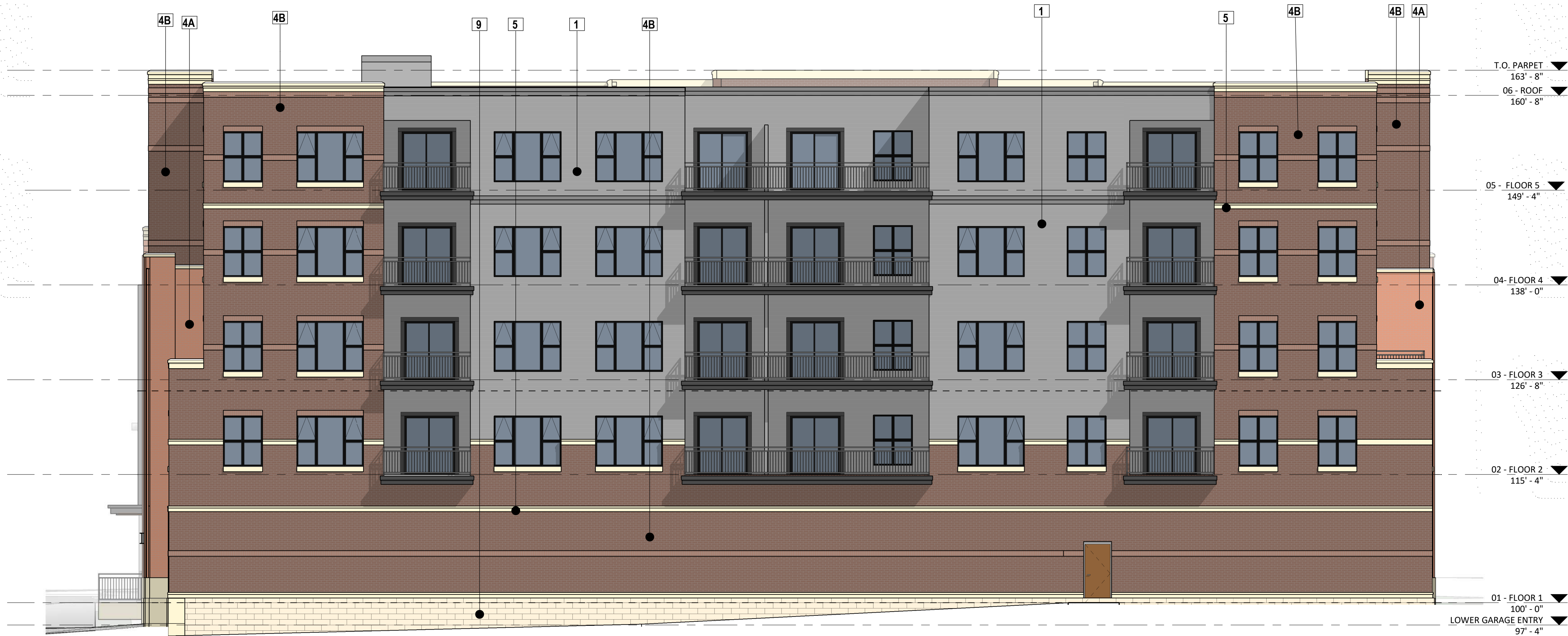
1 NW ELEVATION- COLOR A2.4 1/8" = 1'-0"
