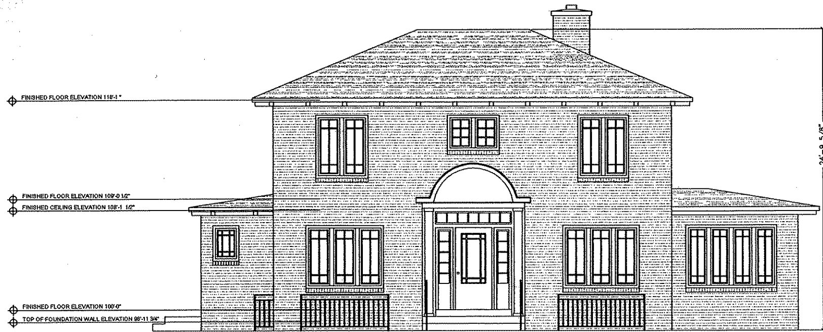
EXISTING WEST EXTERIOR ELEVATION SCALE: 1/8" = 1'-0"
