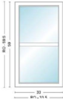
100REC 2' 9"X4' 11", Unit, 100 Series Picture/Transom-PWTR-Insert, No Flange w/Exterior Accessory Kerf (Insert), White Exterior Frame, w/White Interior Frame, Fixed, Dual Pane Low-E SmartSun Standard Argon Fill Full Divided Light (FDL) 1 Wide, 2 High, Specified Equal Light Pattern, White, w/White, 3/4" Grille Bar, Wide Grille Bar: 2 1/4" with Centered Horizontal Bar Placement Stainless Glass / Grille Spacer
