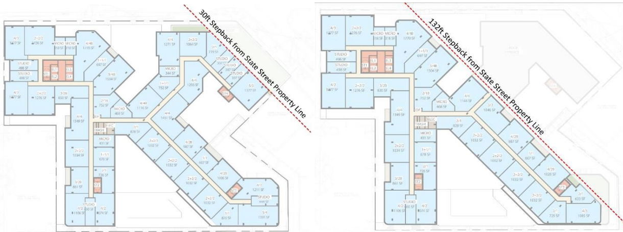
Images 2 & 3: Compliance with the Downtown Plan’s required building height setbacks: (Left) The fourth floor plan’s compliance with the 30-foot building setback from the State Street Right-of-Way above the fourth floor. (Right) The seventh floor plan’s compliance with the 132-foot setback from the State Street Right-of-Way above the sixth floor.
