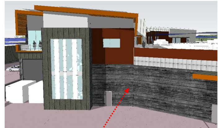
Precast Wall Panels
