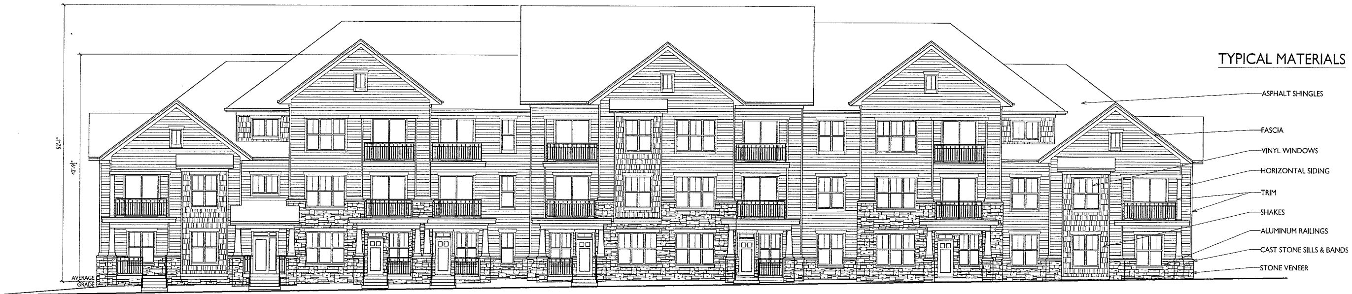
2 WEST ELEVATION (ALONG CITY VIEW DR.) A-2.1 1/8"=1'-0"
