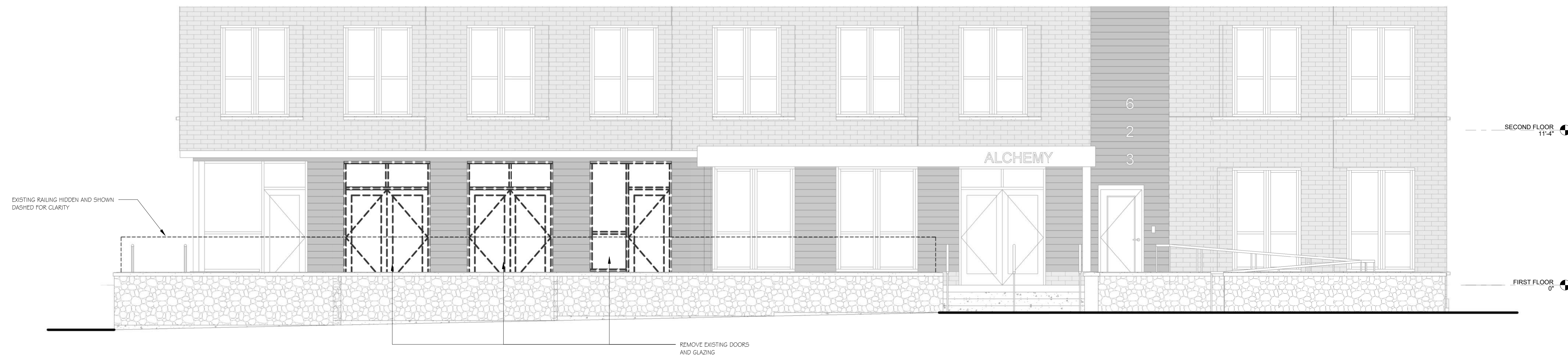
1 WEST ELEVATION (EXISTING CONDITIONS & DEMOLITION) 1/4" = 1'-0"
