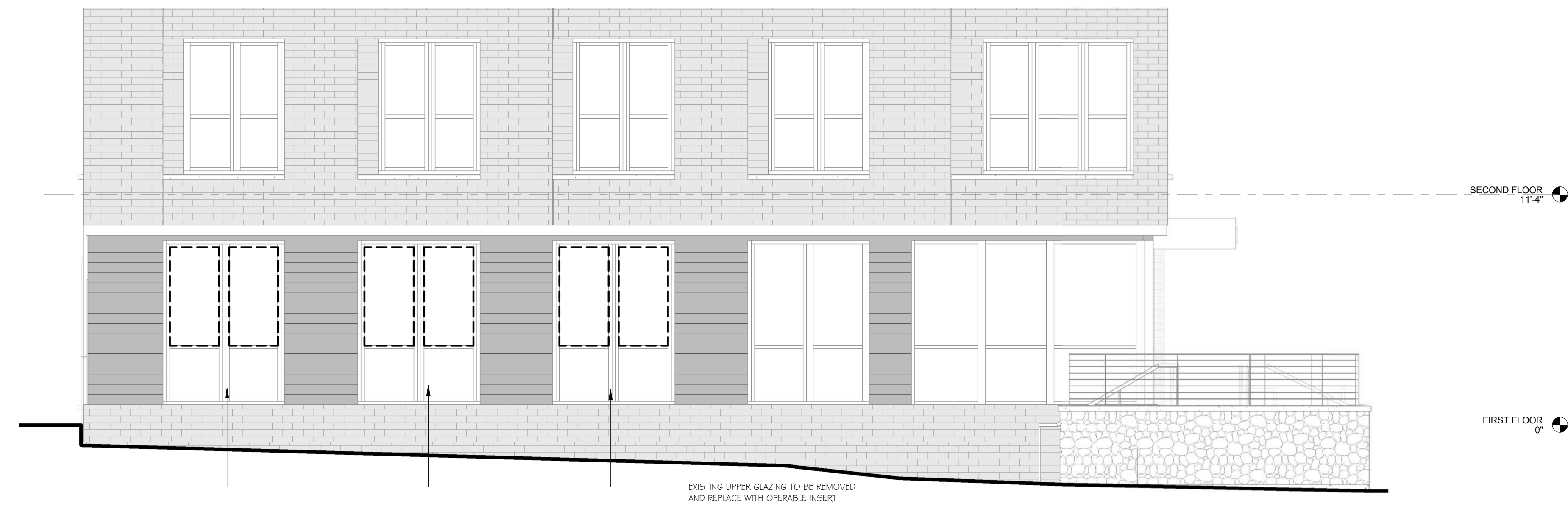
① NORTH ELEVATION (EXISTING CONDITIONS & DEMOLITION) 1/4" = 1'-0"
