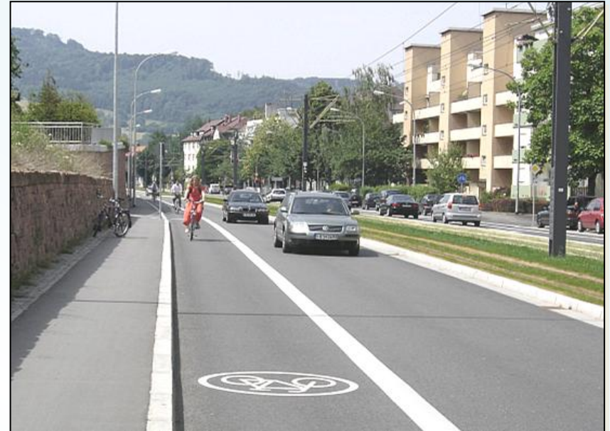
cycle lane on the carriageway next to motor car traffic
