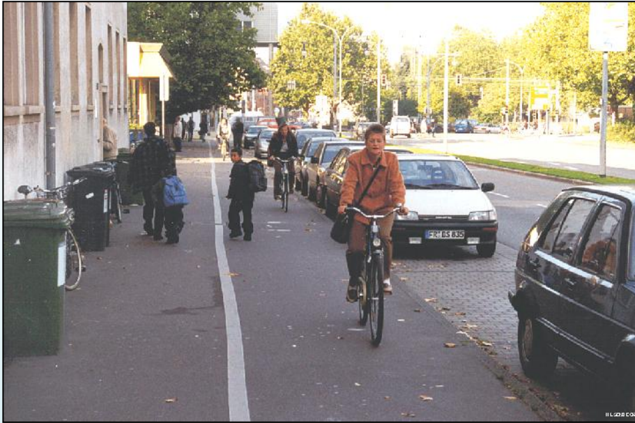
cycle lane between sidewalk and parking lane / motor car lane
