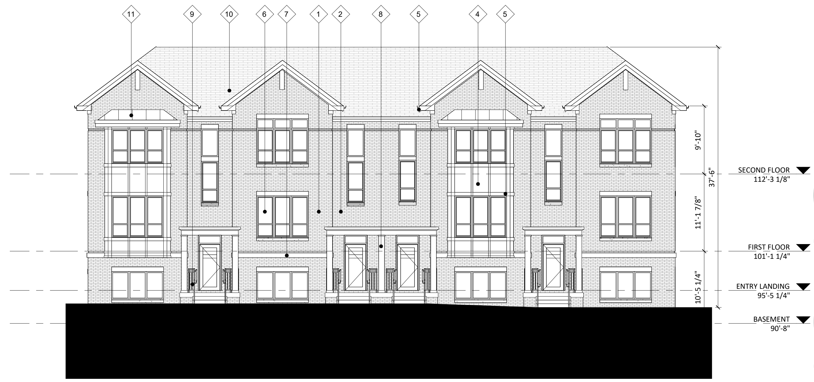
2 ELEVATION - NORTH A-2.1-3 1/8" = 1'-0"
