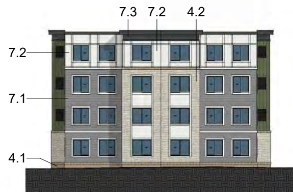
⑤ Bldg B Elevation 5 1" = 30'-0"
