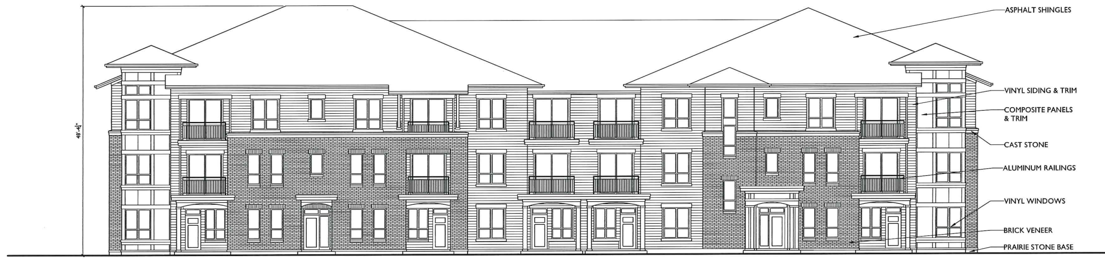
2 NORTH ELEVATION A-2.3 SCALE: 1/8"=1'-0"
