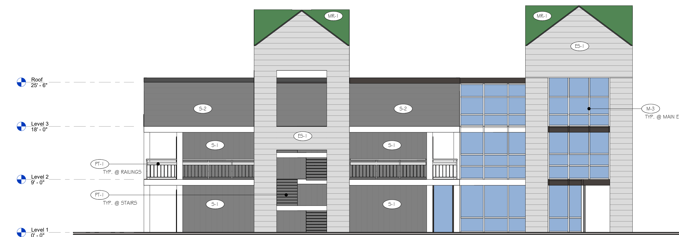
WEST ELEVATION - PROPOSED SCALE: 1/8" = 1'-0" 0' 4' 8' 16' 24'
