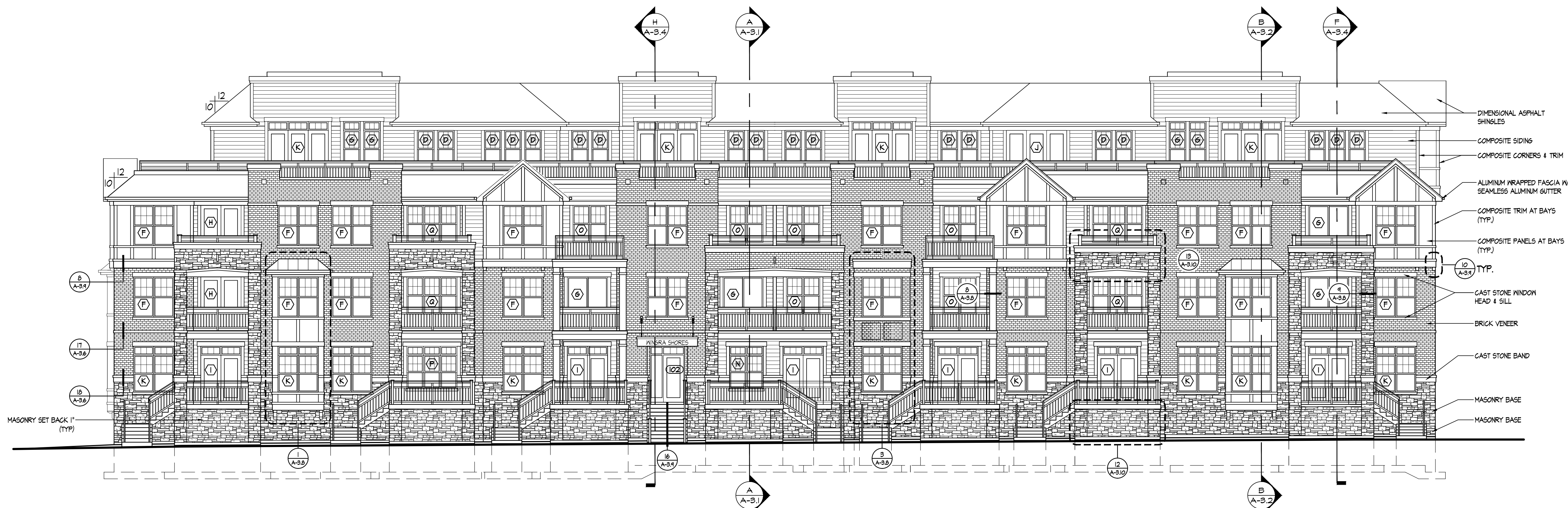
B SOUTHEAST ELEVATION (ARBOR DRIVE) 1/8" = 1'-0"
