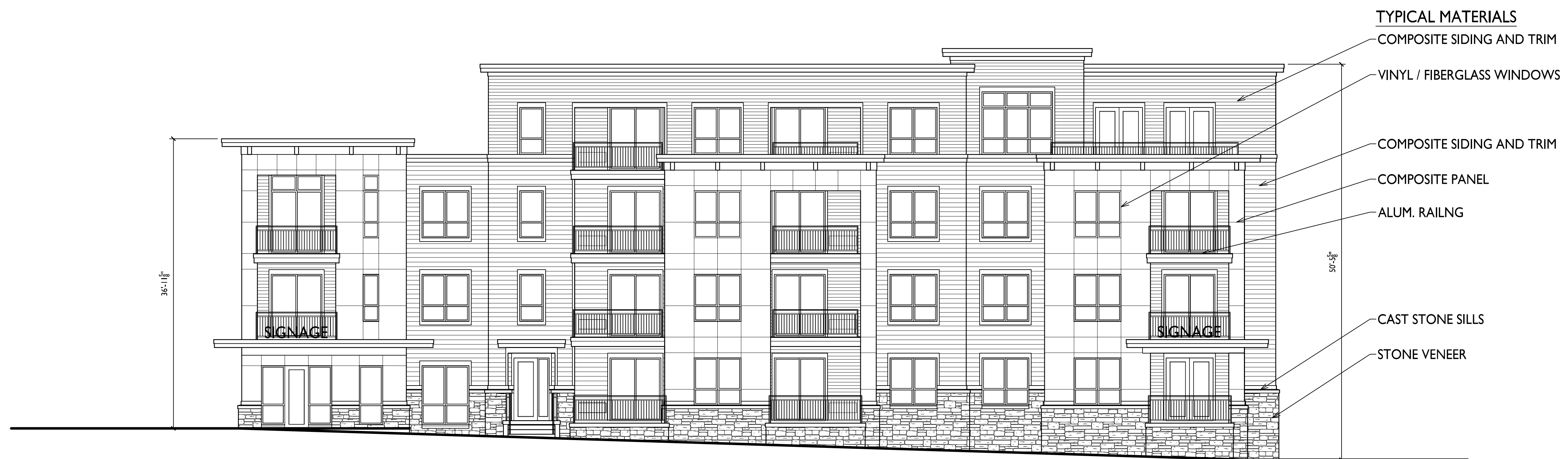
2 A - SOUTH ELEVATION ALONG TENNYSON LANE A-2.1a 1/8" = 1'-0"
