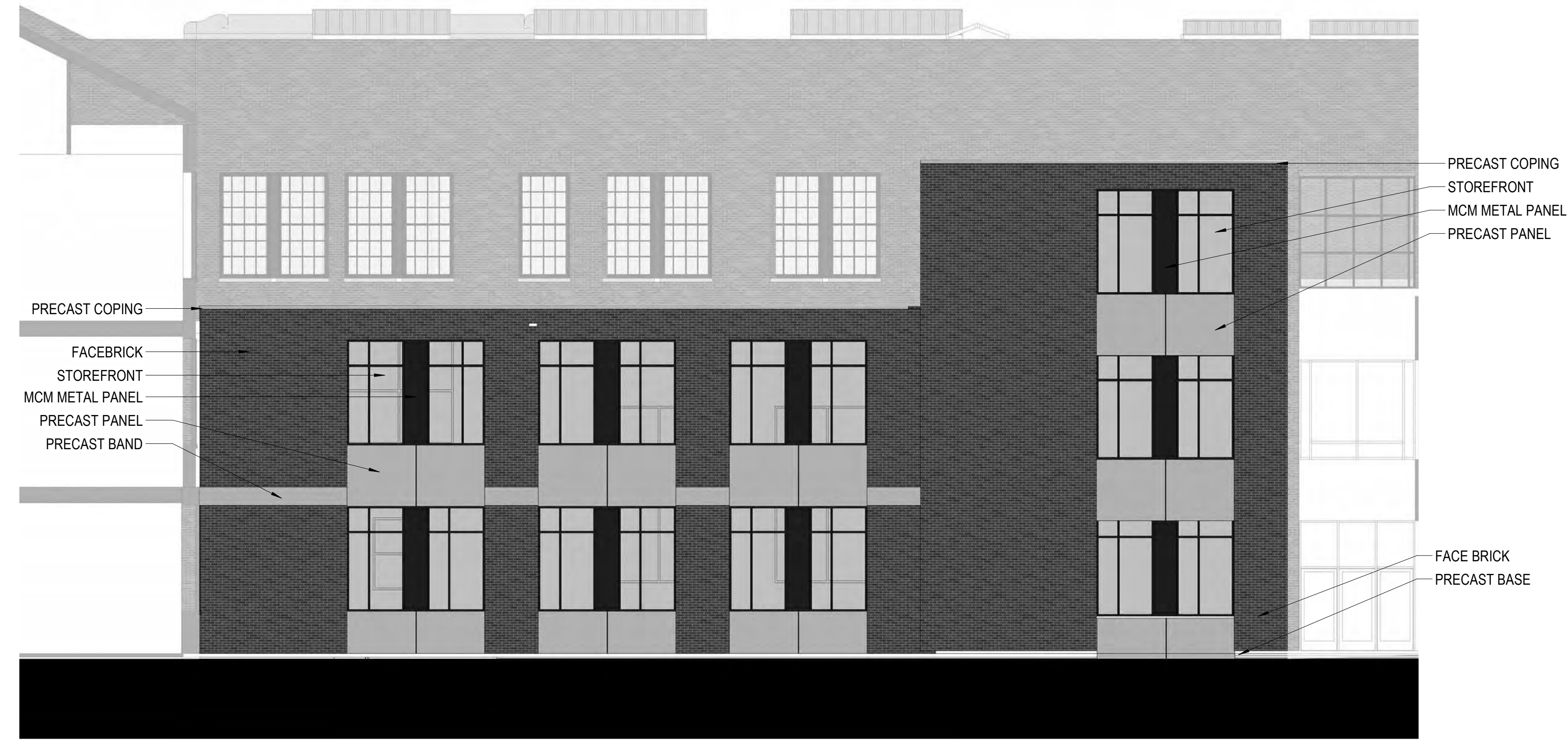
D3 CIRCULATION ADDITION - NORTH - UDC B&W 1/8" = 1'-0"
