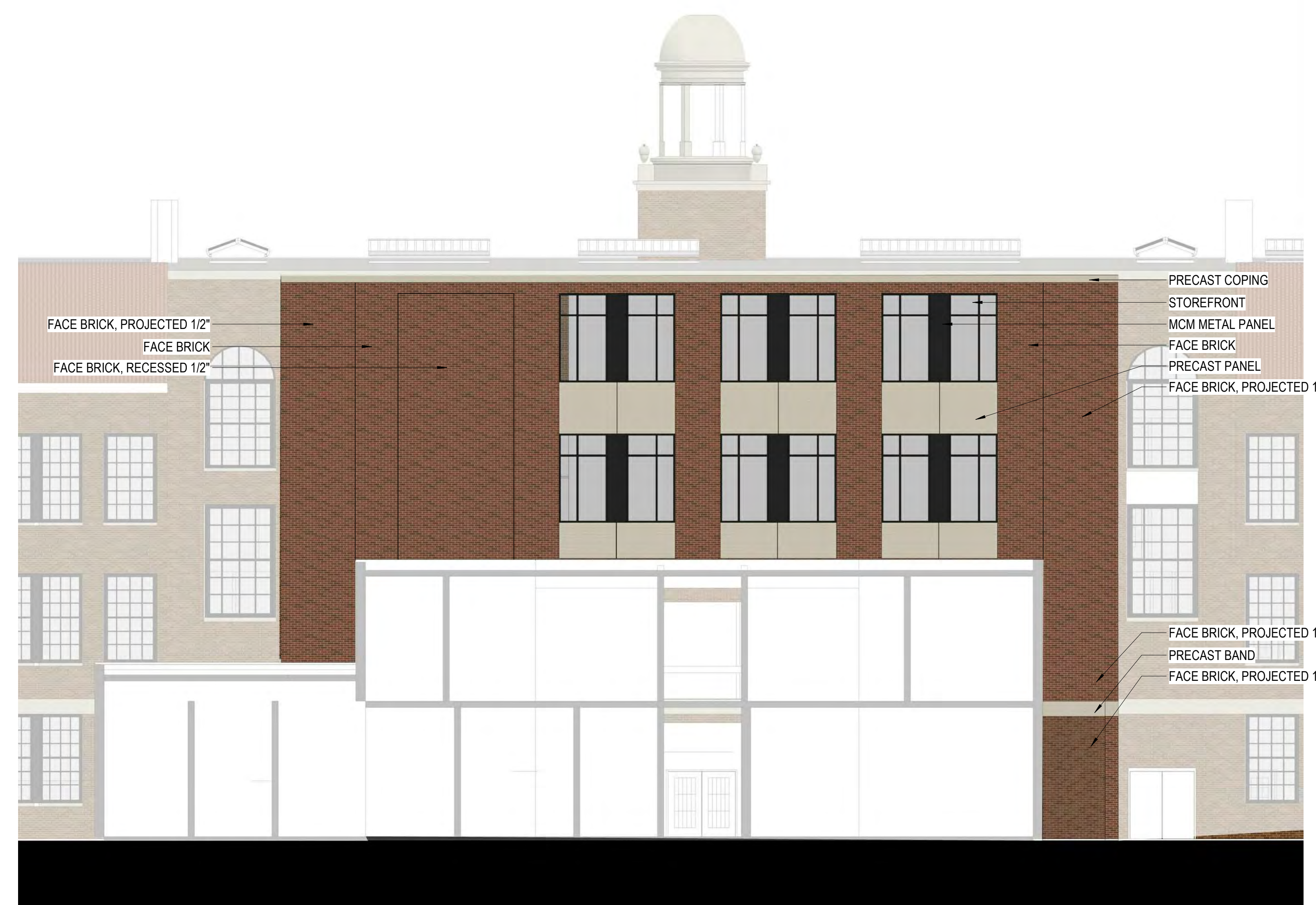
A3 ELEVATOR ADDITION - WEST - UDC 1/8" = 1'-0"
